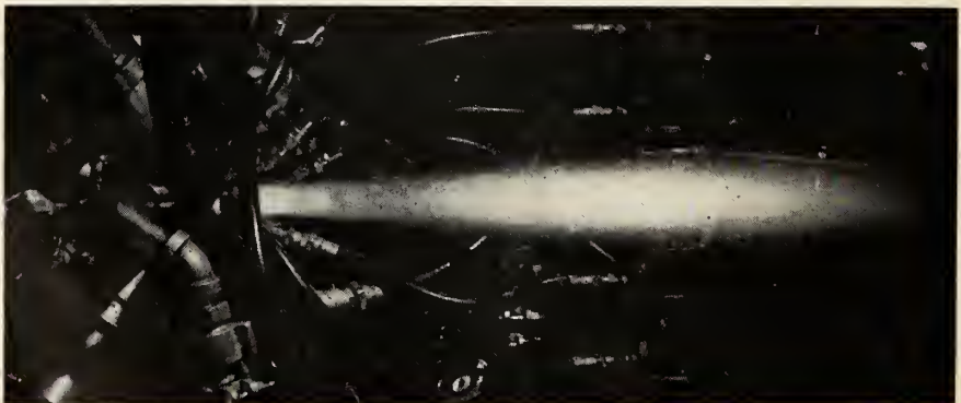
TEN MEGAWATT arc jet in operation. The jet, containing five to six million watts of energy, issues through supersonic nozzle.
