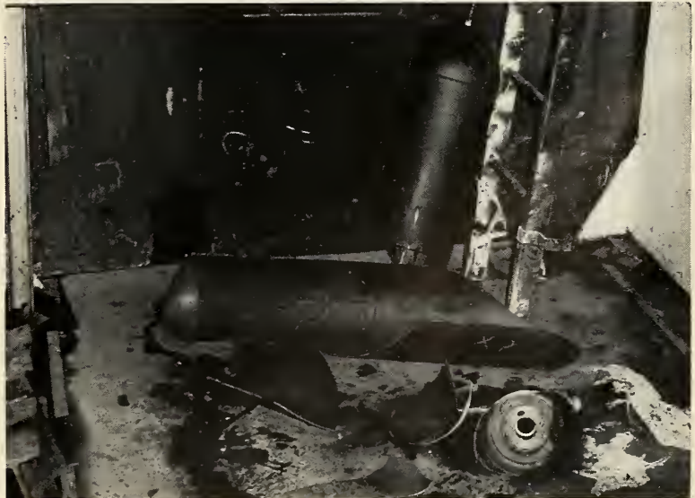
HERE IS an excellent example of brittle failure during hydrotest of a solid rocket motor case. Failure in this case was at less than one-half the values of the tensile coupons that accompanied the chamber through heat-treat. It burst at 1000 psi hydro pressure. The material, a 5% chrome hot-worked die steel, exhibits all the characteristics of a notch-sensitive failure.
