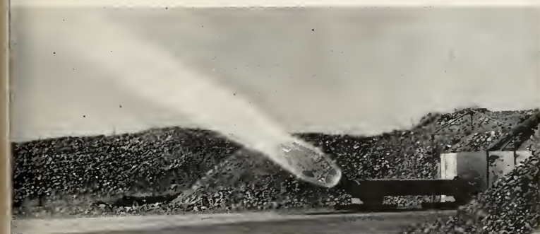
BEST FIRING by Aerojet of large solid-propellant rocket engine for guided missile launches. The company is working on the solid propellants for the Navy's Polaris .
