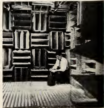
ANECHOIC chamber at CBS Laboratories, Stamford, used for quantitative checks.
