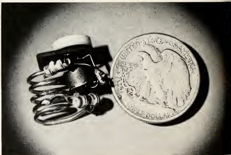
COMPLETE transmitter, no larger than a half-dollar, contains one variable and two fixed ceramic capacitors, a coil, and tunnel diode (in "can" at center of device)
