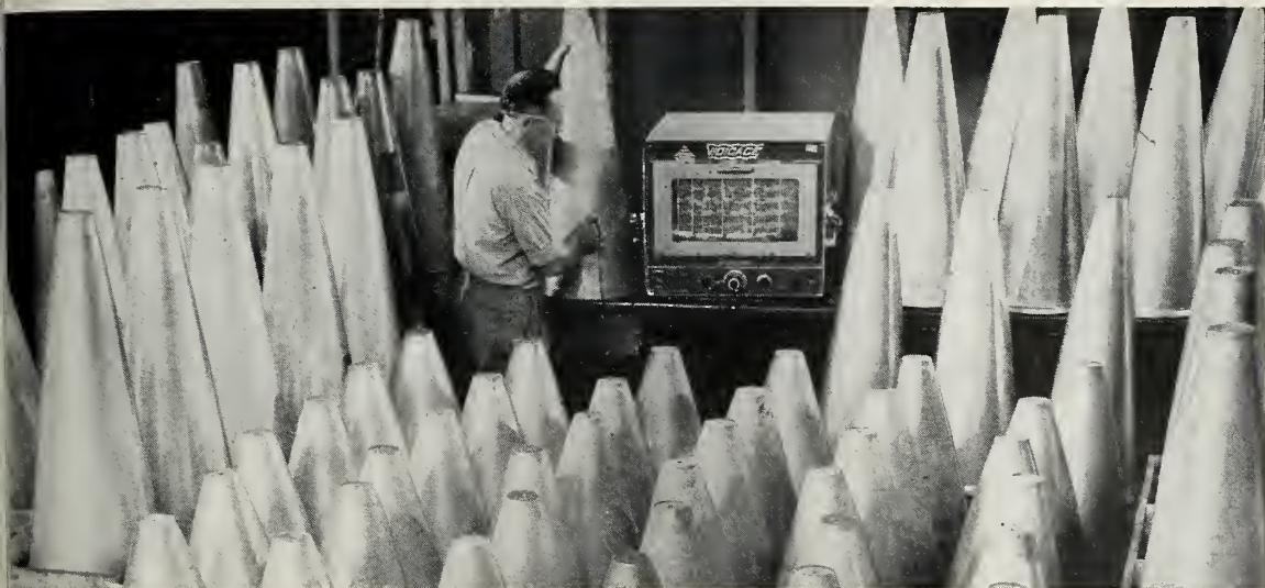
EXAMPLE of inter-industry cooperation in Connecticut is use of ultrasonic resonance gage developed by Branson Instruments, Inc., of Stamford, to test wall thickness of Nike-Hercules nose cones built by Avco's Lycoming Division, Stratford.
