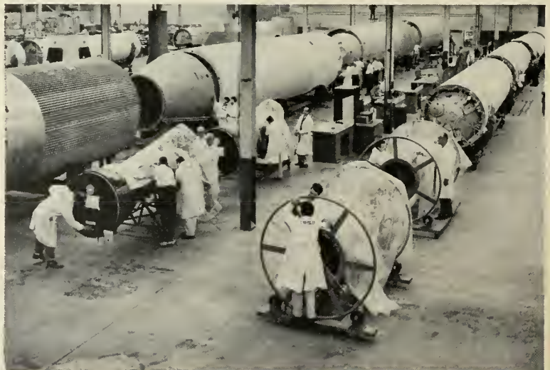
CHRYSLER-OPERATED U.S. Army Michigan Ordnance Missile Plant near Detroit turns out Jupiters and Redstones on parallel production lines employing 10,000 workers.
