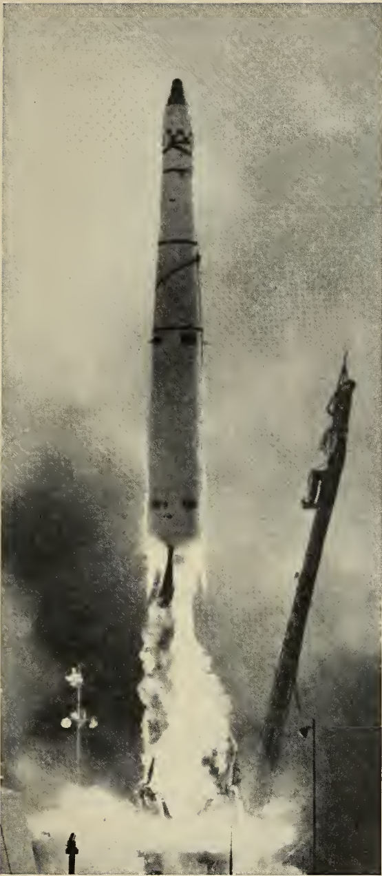
Boosted into space by the 150,000-pound thrust of an Air Force Thor missile, the second-stage Agena satellite is powered into orbit by its own liquid-fuel rocket engine of 15,000 pounds thrust.
