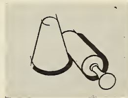
MISSILE PARTS FROM INERT MATERIALS include newly developed asbestos-phenolic compound for nozzles . . . nose cones of fluorocarbon plastics.
