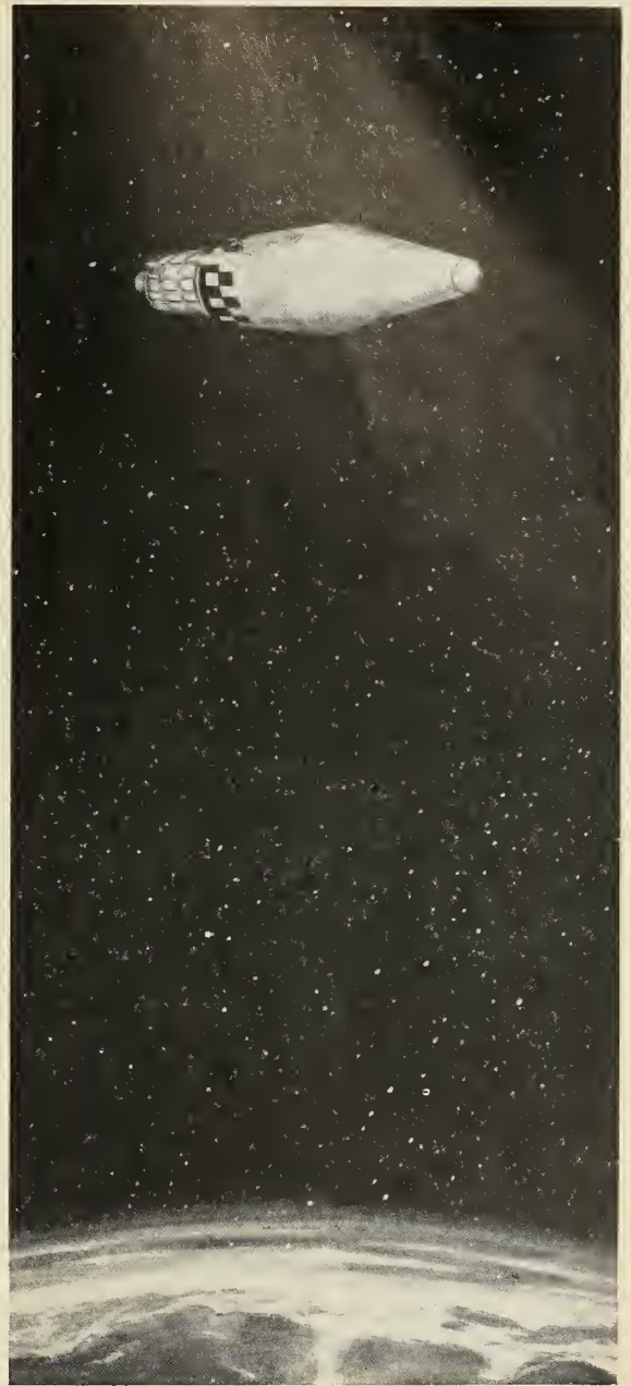
Once in orbit , the Agena satellite radios back to its tracking stations more than a hundred measurements of its performance and of the conditions it encounters as it circles the earth at 18,000 mph.
