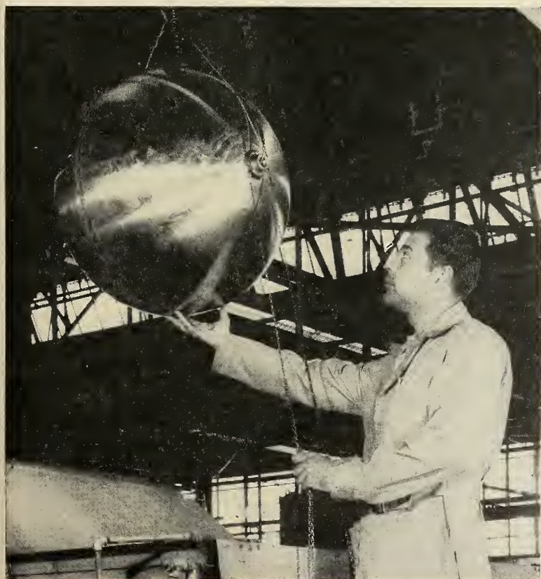
FIRST TITANIUM used on a large scale for missiles was this 50-pound helium bottle in Convair Atlas . Aluminum bottle would have weighed 80 lbs., steel 125.
