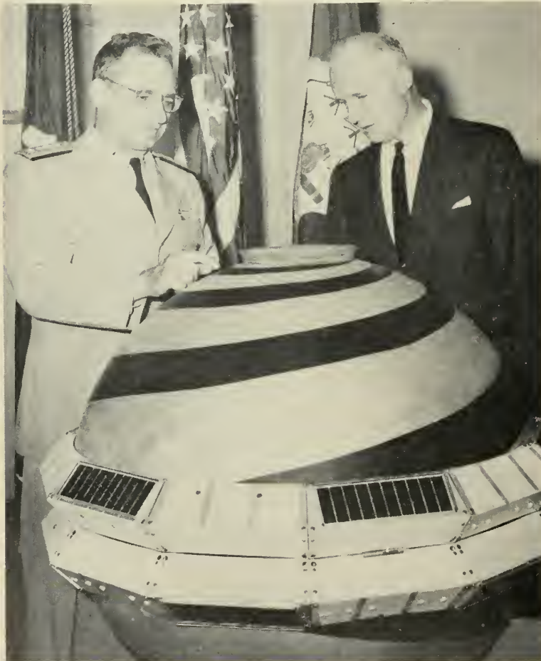
R&D Transit is more than five times the size of planned operational models, to provide redundancy. Antennas are painted on its skin, and its waist is girdled by 12 banks of solar cells. Rear Adm. K. S. Masterson, Deputy CNO for Development, and James H. Wakelin, Jr., Assistant Navy Secretary for R&D, examine satellite.
