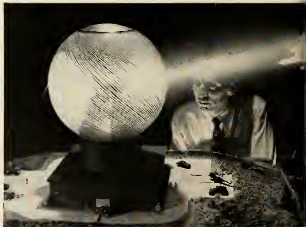
NON-ROTATING 360° RADAR ANTENNA. Only the feed point moves. Principle involved will permit economical construction of very large high gain scanning antennas. Application of inflation techniques will permit lighter-weight long-range air-transportable radar. Working models already built and evaluated. Electronics Division and Research Laboratories
