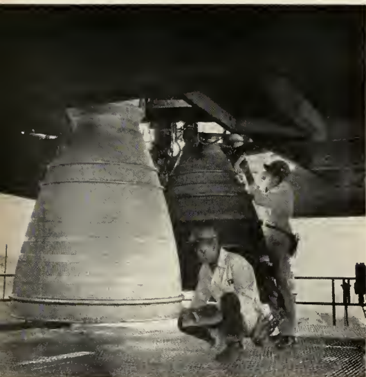
FINAL CHECKS on the Atlas main engine cluster are conducted by technicians at the Propulsion Field Laboratory of Rocketdyne. During 1958 Rocketdyne conducted 4,085 large engine tests.
