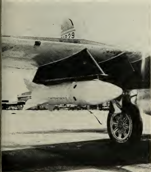
Genie , MB-1, rocket-powered air-to-air missile with nuclear warhead capability is positioned under the wing on an F-89. Missile is also carried in special weapon bays of the F-101, F-102 and F-106.
