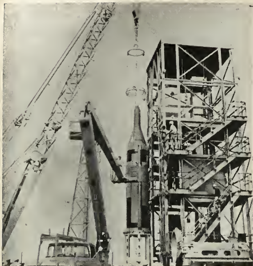
Polaris AX-4 is positioned on launching pad at Cape Canaveral prior to its Jan. 19 firing. Missile is transported to site by a trailer erector. Crane then lifts it to top of pad.
