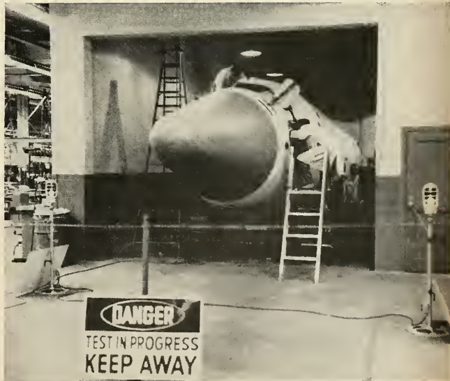
FACTORY TEST of the Jupiter IRBM at the Army Michigan Ordnance Missile plant, operated by the Chrysler Corp. The plant which produces Redstone and Jupiter missiles on parallel assembly lines, has 2.1 million square feet of floor space.
