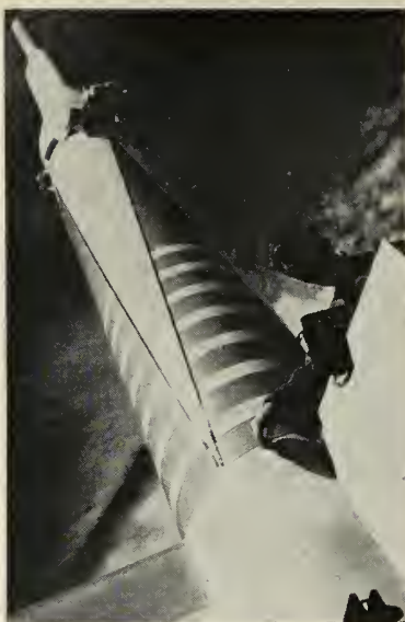
X-17 WAS FIRST ballistic missile to prove nose cone could survive re-entry of Earth atmosphere.
