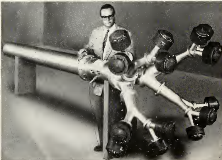
ALTEC LANSING Corp. has developed a 155-db 8-inch plane-wave tube to observe and determine electronic equipment malfunctioning in missiles.
