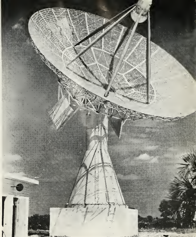
RADIATION/KENNEDY CO. TLM18 automatic tracking telemetry antenna has rates of over 7°/sec.
