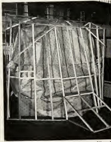
PART WAY , the boring mill is covered with protective paper and frame.
