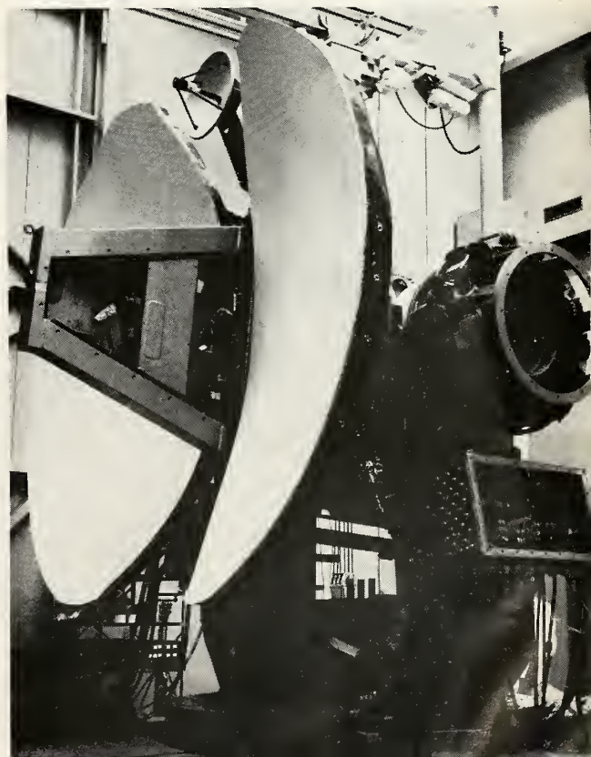
GE's high-precision Atlas tracker theoretically is accurate enough to measure an angle of one foot at 25 miles.
