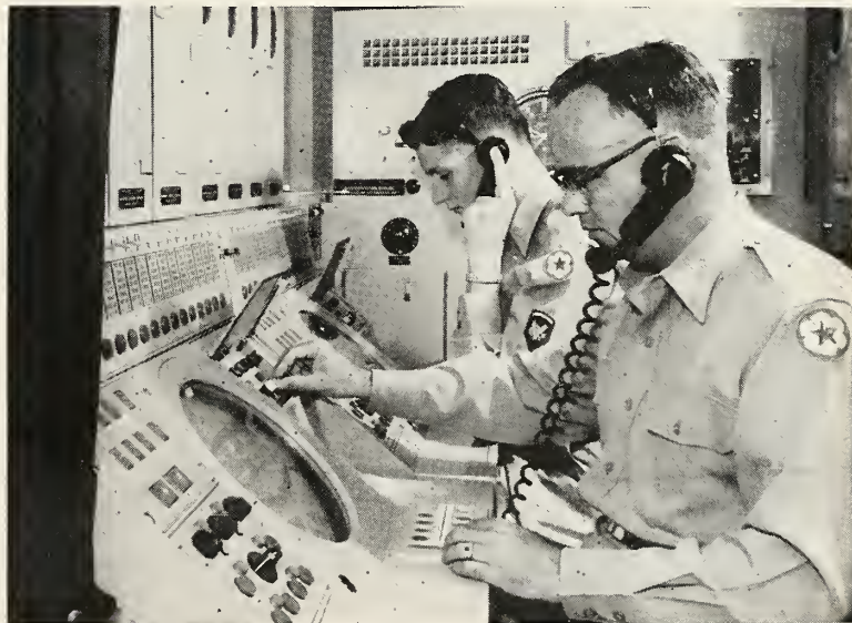
"VEST POCKET" DEFENSE against enemy jets is provided by the Army's new mobile tactical air defense system. The system—developed by Hughes Aircraft—is capable of semi-automatic direction of the firing of from one to eight Army anti-aircraft and missile batteries. Several of the five-truck systems are already in the hands of U.S. troops in Europe for use with Western-Electric Nikes and Raytheon Hawks.
