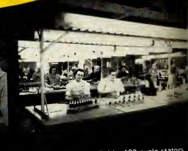
Winding armatures, fields, 400 cycle stators
