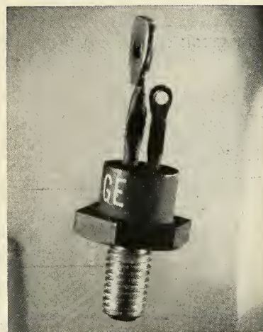
GE's solid-state thyatron can switch kilowatts of power in microseconds.
