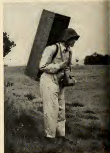
CONTAINER with two missiles weighs only 23 lbs. and is strapped on back missiles and rockets, June 1, 1953
