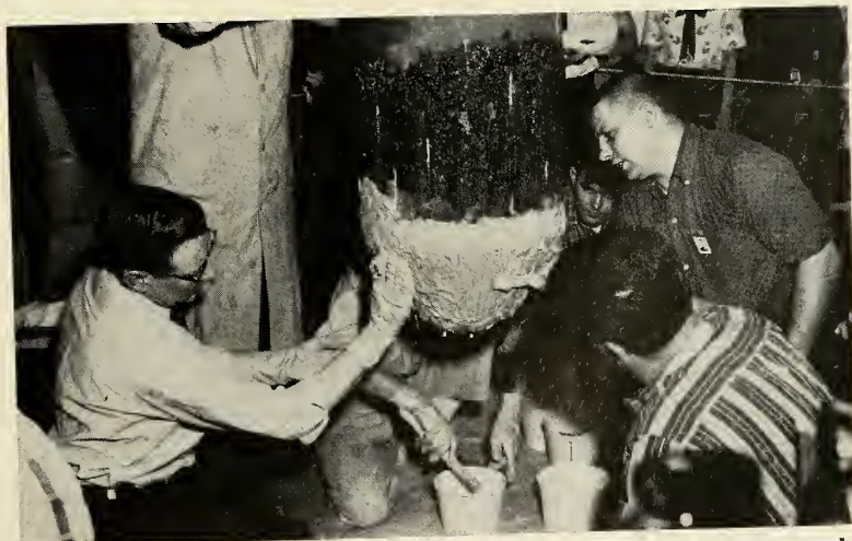
TECHNICIANS coat nose cone of Thor-Able re-entry vehicle with plaster to make cast of its surface. Vehicle is first to be recovered after successful flight over 5000-mile ICBM distance. Avco's Research and Advanced Development Division developed ablating heat shield material which protected cone from extreme temperatures encountered during re-entry into earth's atmosphere. (Dark substance behind cone is ablative material which flowed back over main body during re-entry heating.)
