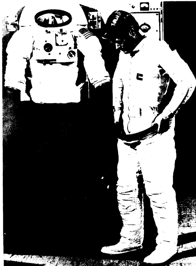
SHUTTLE SPACE SUIT - Space Systems engineer Ed Brisson models the undergarment that will cool and ventilate Space Shuttle astronauts when they wear the Shuttle Extravehicular Mobility Units. Excess body heat is removed by water circulated through the thin plastic tubing woven into the fabric and by oxygen carried through hose-like tubes. Brisson has slipped into the lower portion of the suit.
