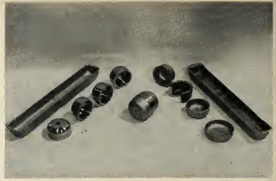
RECTANGULAR PIECES are "boats" for containing small parts in furnaces, and round cups could be gyroscope rotors.
