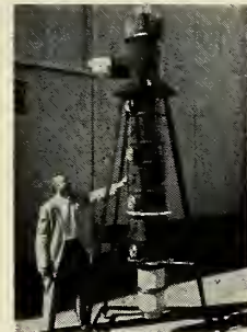
VARIAN Associates has developed this 12-foot, 900-pound klystron tube for missile tracking.
