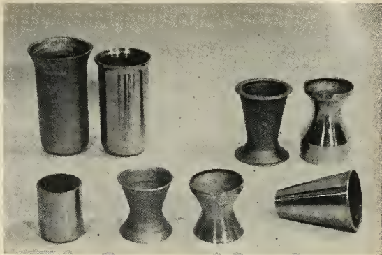
PARTS FABRICATED from tungsten sheet by spinning, an art dating back to Middle Ages but new to refractory metal.
