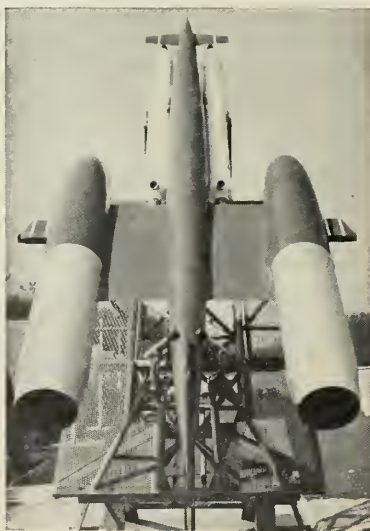
NORD AVIATION'S CT-41 target missile will be made under license in Britain by Hawker-Siddeley. The supersonic bird has two wingtip-mounted ramjets and is controlled from the ground.
