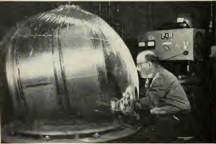
Welding of titanium at P&WA is based on the company's experience in production of more than 5800 jet engines containing titanium parts. Weld strength of beta titanium alloy is considerably improved by cold working the weld.
