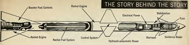
**THOUSANDS OF "FAULTS"** can develop in a guided missile, each capable of causing it to misfire or swerve off-course. Pre-launching
