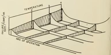
Figure 3. Effect on component failure rate by increase in temperature.
