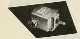
The linear actuator below, was designed and built to provide reliable electrical actuation in an environment of violeot centrifuging and vibration. This unit weighs less that 1.5 pounds, yet is capable of operating against opposing loads of over 100 times its own weight.
