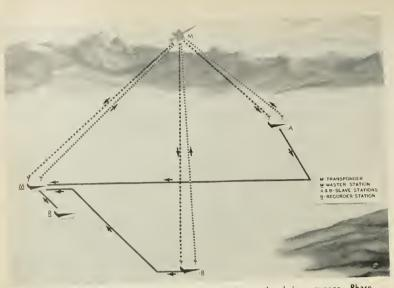
Phase measuring system. Stations send and receive a signal in sequence. Phase shift is proportional to change in path length. Station gets independent readings.
