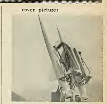
Oerlikon's type 54 SAM, over 19 feet long, is regarded as one of the world's best antiaircraft missiles. The type 54 is a beamrider and utilizes a liquid propellant engine burning white fuming nitric acid and kerosene. The beam-transmitter of the type 54 system is shown on the cover of missile electronics (following page 156) and has both coarse-beam and fine-beam guidance.
