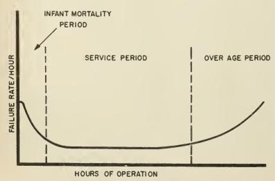
Figure 1. Component failure rate vs. operating time.
