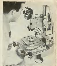
Gaertner Toolmakers' Microscope used to measure typical piece part. Co-ordinate range 4" x 2".
