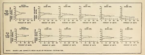
Figure 5. Per cent deviation in component characteristic for operation at 100 per cent and 50 per cent of rated load.
