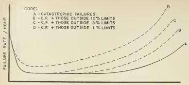
HOURS OF OPERATION Figure 2. Component failure rate per hour.
