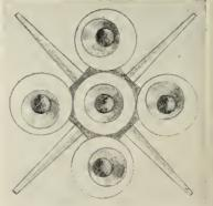
Aft view of the booster section of a possible arrangement for a 1500-mile POLARIS test missile. Center rocket could either be second stage of three-stage configuration or fifth booster rocket of possible two-stage model.
