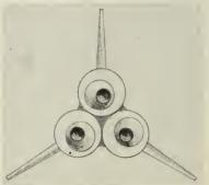
Aft view of possible arrangement of an 800mile POLARIS test vehicle. Three solid-propellant rocket motors with canted nozzles arranged to impart spin during boost.
