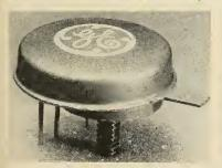
temperature transistor in the industry. The device will dissipate 85-watts at  $25^{\circ}$ C mounting base temperature and has a nominal collector saturation resistance of 2 ohms.
