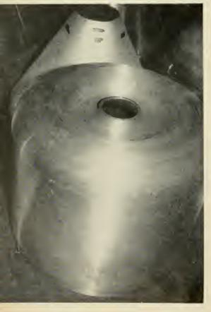
Right, cone of 5%" magnesium, hot spun in two parts on LEICO Model PIb 1200. Previous to new method, welded heavy or thickwalled parts caused warpage which in turn required an inside and out operation. The machines are now being used in many parts of U.S.A.
