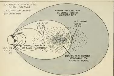
Fig. 6. Radiations in the Outer Ionosphere (controlled mainly by earth's magnetic field)
