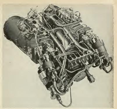
Detailed picture of Napier Double SCORPION NSc. D.I. used to attain the altitude in a Rolls Royce Avon-powered CANBERRA. It is a double-barreled version of the NSc. I rocket.
