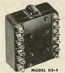
Triple-Pole, Double Throw 15 AMP, 125/250 V. A.C. 30 V., D.C. Res. 10 AMP, 30 V., D.C., Ind. Overtravel, .015 Min. Move. Diff., .028 ± .007 Mech. Life, 1.000,000 ops. Elec. Life, 500,000 ops.
