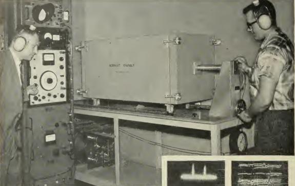
L to R: Dr. Fricke, Engineer-in-charge Acoustics Laboratory, and Mr. Kuzara Acoustics Engineer, evaluating a component in a high intensity acoustic environment. RIGHT: Malfunction of a relay at bigh-intensity sound as disclosed in a sound chamber.
