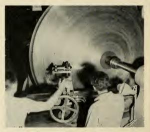
Cold spinning 5%" aluminum alloy to an 8' finished part for ICBM pressure bulkhead. Used here is Model PIb 1200 hydraulic spinning and planishing lathe. German manufacturers are Leifeld & Co.
