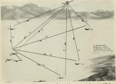
Radar triangulation pulse time system. Pulse-modulated carrier is frequency shifted in missile. This signal is again shifted by slave stations and sent to master station.
