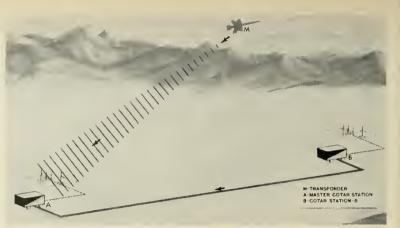
Interferometer system similar to MINITRACK, using two stations to measure phase difference at multiple antennas. Two-station system gives position, velocity, acceleration.
