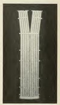
Complete afterburner cooling assembly. Note use of straps to gang the tubing.
