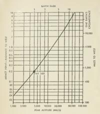
Fig. 4. Relationship of a altitude to impact point.
