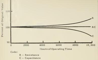
Figure 6. Drift trade-off in R-C circuit.
