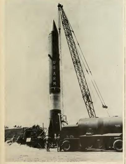
A REDSTONE missile, with frost forming on its skin from the liquid oxygen in the tanks, stands ready for launching. Note the logistical field support equipment that is now operational.
