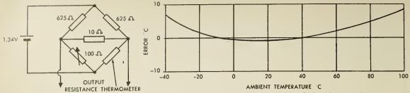
Fig. 3-Circuit diagram of "zone box" and graph illustrating the error of improper tracking of the reference thermocouple output.
