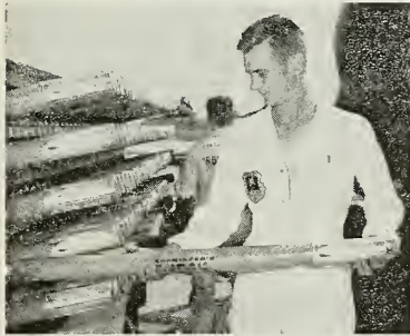
Careful handling of the 2.75-inch rockets is necessary to prevent cracks in the propellant which could cause uneven burning or even premature burnout. Metal cans ground the firing mechanism to prevent accidental ignition.
