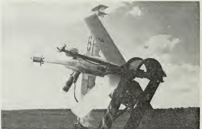
DART is wire-guided, praised for simplicity, accuracy and ease of handling. Design is based on German and French concepts; Germans used wire-guided missiles in the last war.
