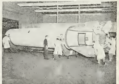
Huge missile is transported on special dollies; weapon is designed to take rough handling and transportation.
