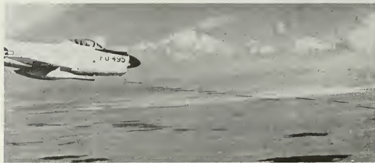
North American F-86D all-weather interceptor launches a stream of 24 2.75-inch rockets at a tow target high over the Arizona desert near Yuma. Note retractable rocket launching tray beneath cockpit.
