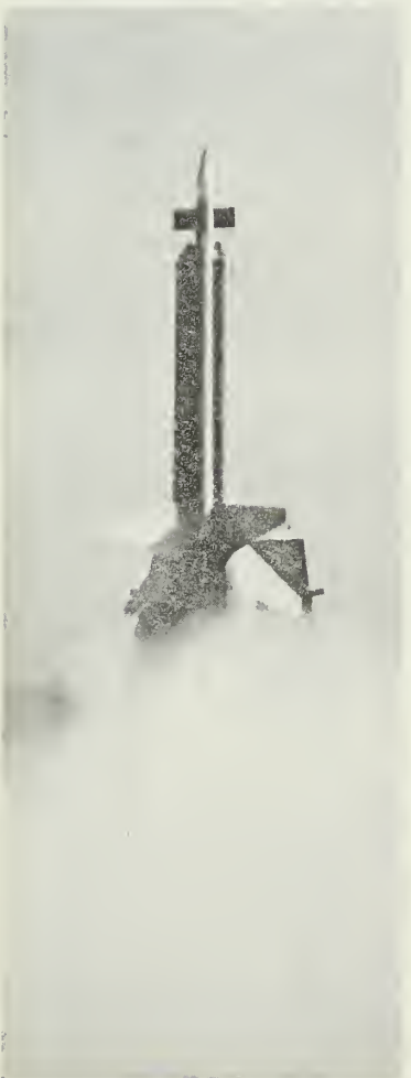
Simple NACA model to check operation of a new multi-rocket booster.
