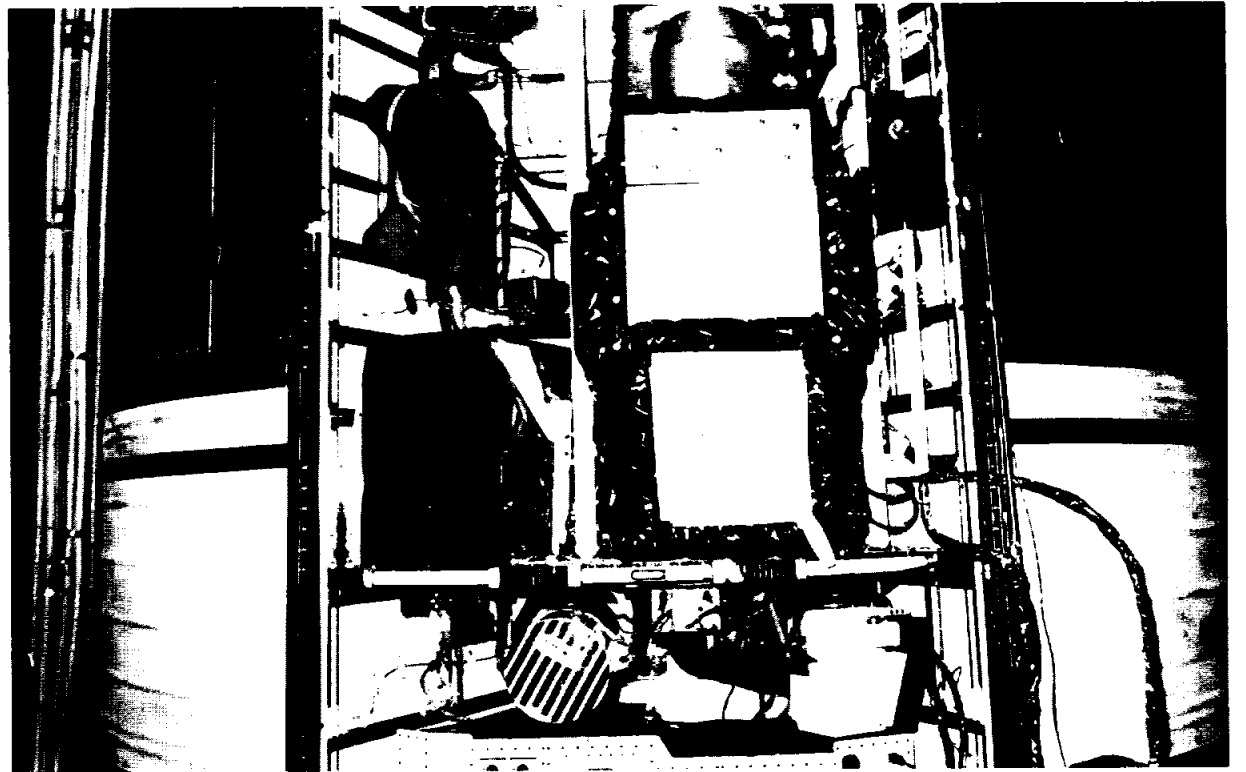
SIM MODULE —Pictured here is the J-Series Apollo Scientific Instrument Module which occupies one bay or 1/6 of the 2TV-2 service module. This particular SIM is configured for Apollo 15. It contains a laser altimeter, subsatellite experiment to be placed in lunar orbit; mass, gamma ray, x-ray, and alpha particle spectrometers; and two cameras, one for mapping and one which will take panoramic "stereo" pictures of the lunar surface. The Command Module Pilot will perform extravehicular activity to retrieve the film cassettes.
