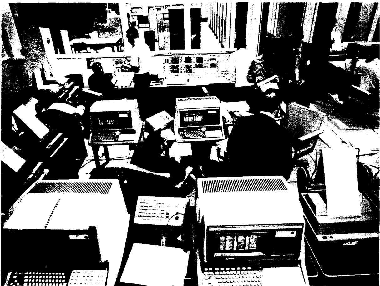
MONITORING —FSD engineers monitor in the Data Control Area of CCATS (communications, command and telemetry systems) to verify the computer is receiving, processing and routing data properly during MCC internal validation last week.
