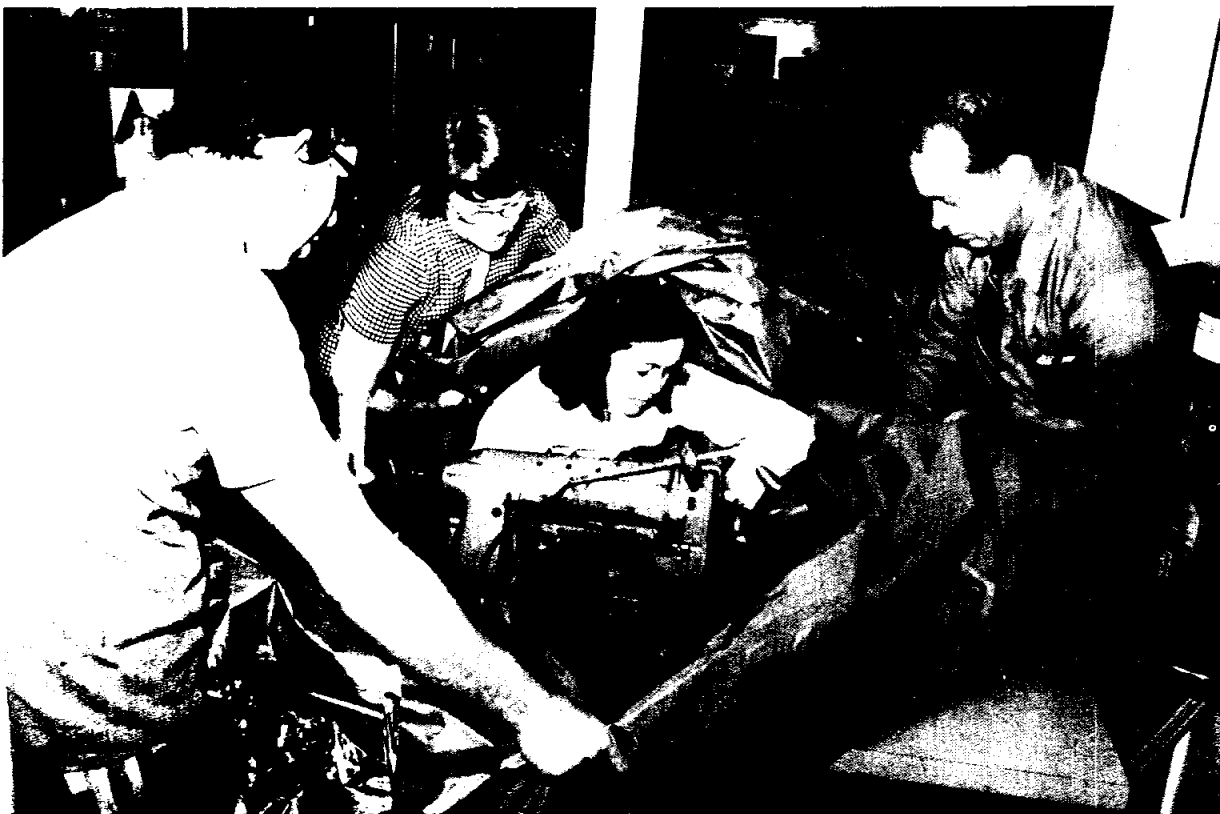
SKYLAB SOLAR SHIELD—A sail-like sunshade for possible use as a sunshield for the Skylab Orbital Workshop (OWS) is shown being fabricated in the GE Building across the street from JSC. The material is being fed through the sewing machine. Working on the sunshade, left to right are Dale Gentry (GE), Elizabeth Gauldin (JSC), Alyene Baker (GE), and James H. Barnett, Jr. (JSC).
