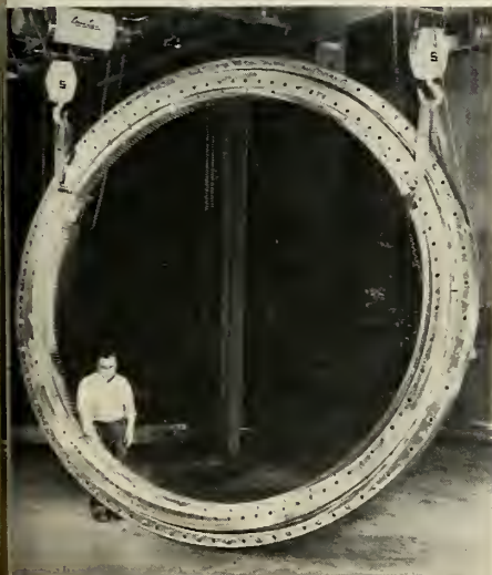
THIS BALL bearing made by Kaydon Engineering Corp. is 13 feet 9 inches in diameter. Designed for the Nike-Zeus radar system, it will hold weight of one-million pounds.
