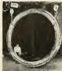
RADAR SYSTEM for Nike-Zeus will require this mammoth ball bearing, supporting million lbs.
