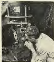
THIS GADGET is providing new measurement techniques at Martin for gyro drift. (See p. 22)
