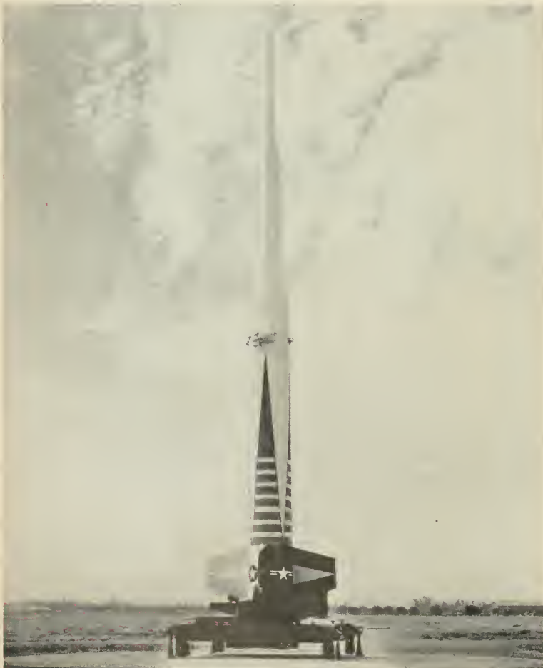
Lockheed proudly displays its X-17 re-entry test missile. Vehicle is said to have made numerous successful flights. Note bulky spin stabilizer rockets mounted on first stage.
