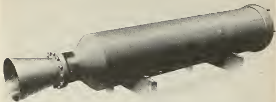
The SEPR-505 solid propellant booster rocket has a thrust of 22,000 lbs. for 4.5 seconds. Weight loaded is 884 lbs. and overall length is 7.9 ft. Chamber pressure is 780 lbs. per sq. in.
