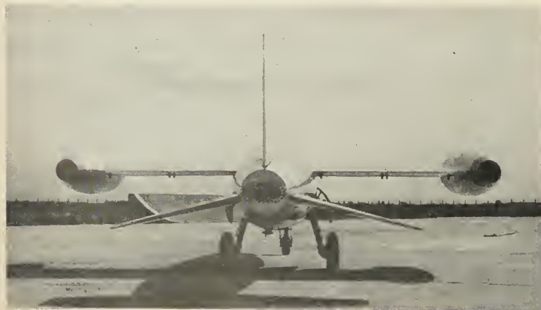
Tail view of the TRIDENT II shows two rocket chambers. TRIDENT I had three chambers.
