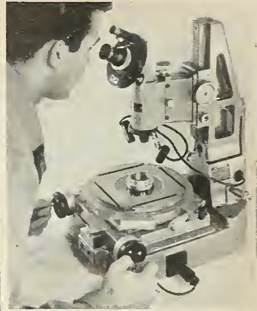
Toolmakers' microscope reads to 0.0001" and 1 minute of arc. Co-ordinate range 4" x 2". Compact built-in rotary stage.
