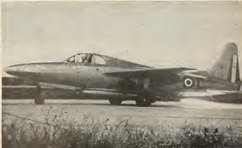
Quest-Aviation's 6025 Espadon was the first French aircraft with rocket power. The SEPR-25 rocket engine of 3,300 lbs. thrust enabled the aircraft to achieve Mach 3 and an altitude of 50,000 ft. Slung under the fuselage is a Rolls-Royce Nene.
