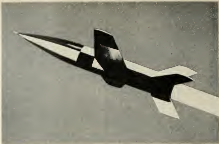
This early Russian missile was powered by a liquid rocket engine. Its launching weight was 3,300 lbs. and its top speed was Mach 1.3. It was 15 ft. long and 24 in. in diameter.
