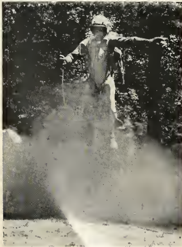
GRASSHOPPER —Reaction Motors Division of Thiokol Chemical Co. has come up with this rocket-powered jump belt which will enable soldiers to leap distances up to 20 ft. carrying equipment to 30% of their own weight.
