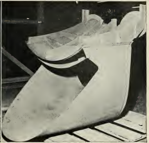
Engine air scoop casting made by R. H. Osbrink Mfg. Company, Los Angeles
