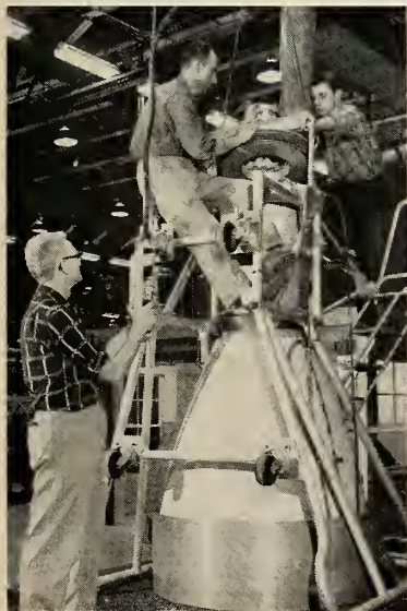
THOR THRUST CHAMBERS are calibrated with 1,000 psi water flow tests before leaving the fabrication area.
