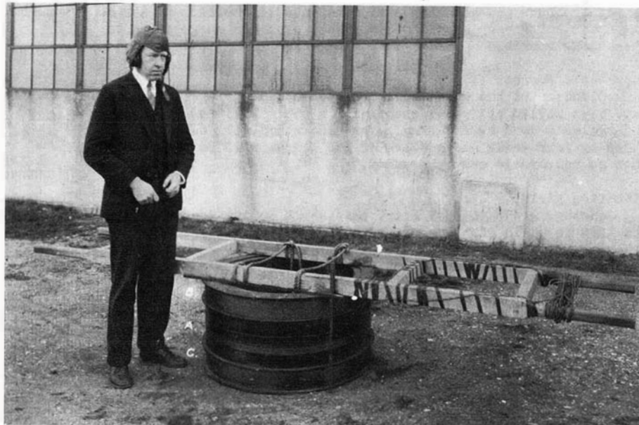
The above picture taken in 1930 shows Gilbert Strailman, Head of Electrical Engineering, with the Laboratory's home-made bomb detector. The site now occupied by the Tank was an ammunition dump back in the old days and when plans were made to erect the Tank there some device had to be rigged up for detecting the bombs that had sunk under ground. Strailman was assigned the job of doing the wiring on the apparatus.
