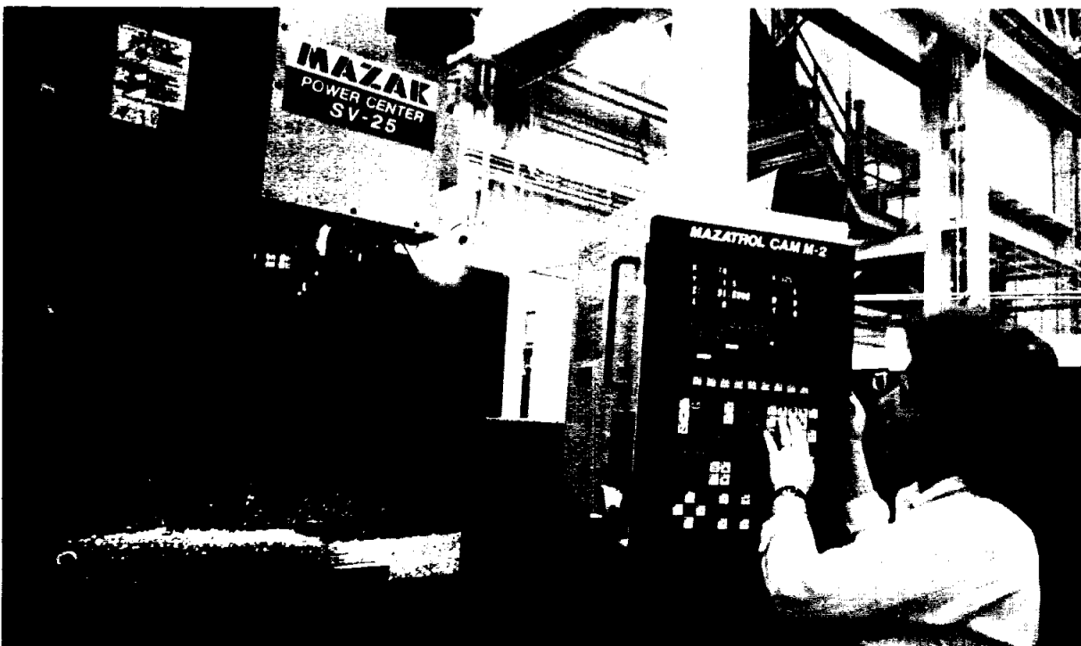
Joyce Davis of Tech Services uses a CAM transmittal to program a metal machining device.
