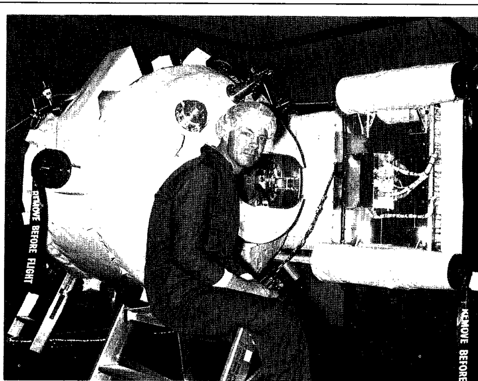
SPAS SITTING — STS-39 Pilot Blaine Hammond inspects the Shuttle Pallet Satellite (SPAS-2) at Cape Canaveral Air Force Station in Florida. SPAS will carry the Infrared Background Signature Survey away from Discovery so that a series of complex rendezvous maneuvers may be attempted. During the maneuvers, the IBSS will examine Discovery's rocket plumes in a sophisticated Strategic Defense Initiative experiment. STS-39 will be Hammond's first flight.
