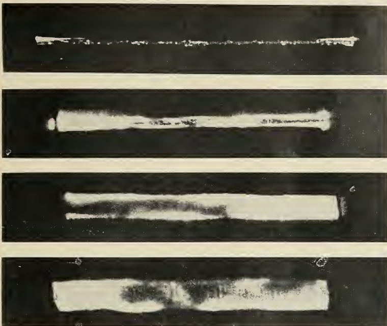
SERIES ILLUSTRATES reaction of exploding aluminum wire 3, 8, 32 and 45 milliseconds after induction of current. Wire was 1 mil in diameter, 3/16" long.
