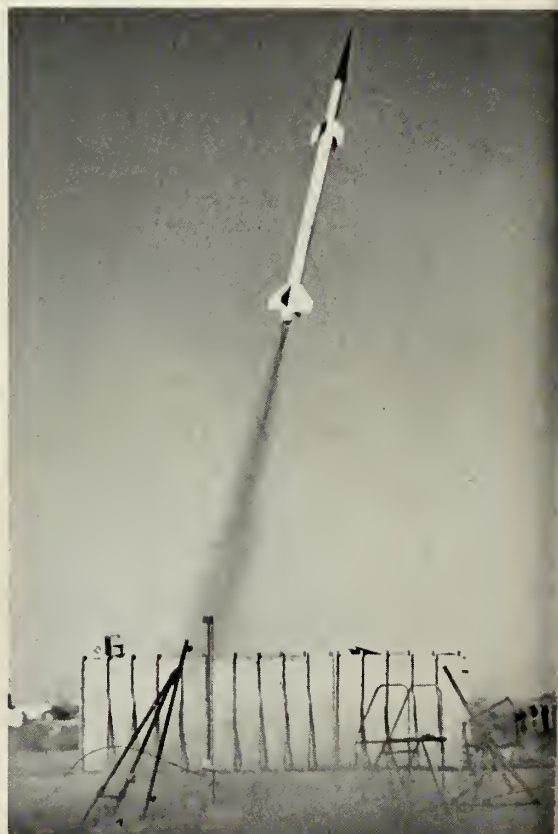
TERRAPIN, named for the slow-moving turtle, streaks skyward at 3,800 mph and telemeters back research data during its 80-mile trip.
