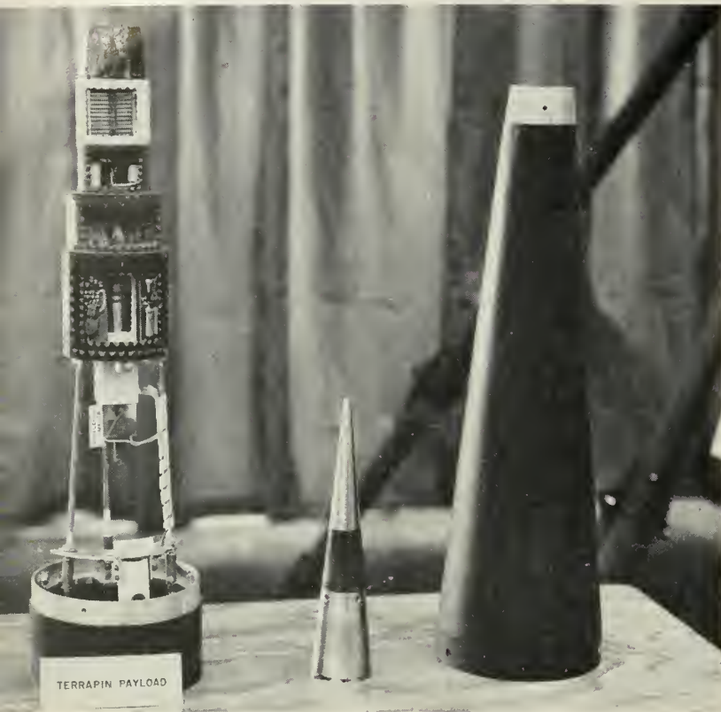
TERRAPIN instrumentation payload including radio transmitting antenna and nose cone. Its nose cone section can be varied in length to accommodate equipment weighing from four to 24 pounds.
