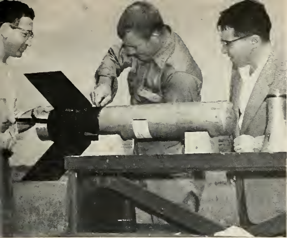
Attaching TERRAPIN'S second-stage rocket engine assembly to second-stage fin section. Left to right: Republic Guided Missiles Div. Project Engineer MORRIS ROTH, NACA's GEORGE CUTTER, and SIDNEY HELFMAN, Republic's Aerodynamics Div. Chief.
