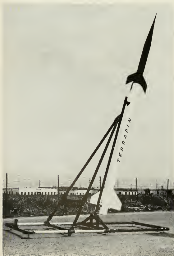
TERRAPIN in its launcher and ready to go. A major design objective was to cut preflight assembly and preparation time to a minimum.
