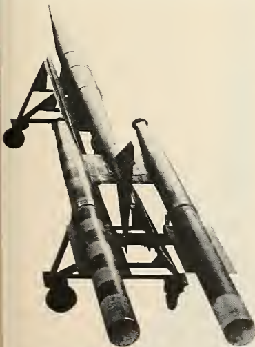
Bristol fitted damping plates to the ramjets in one of its experimental test vehicles to raise the critical flutter speed well beyond that encountered in current operating range.
