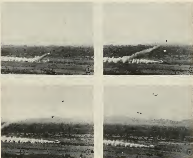
High-speed sequence camera records ejection of two dummies from Convair TF-102A rocket sled at Edwards AFB in California. 1) RESCU Mark I seat, trailing smoke from rocket clears cockpit. 2) M3 cartridge seat (arrow) is ejected as RESCU Mark I rocket burns out. 3) Rocket seat follows trajectory well above M3 seat. 4) Dummies separate from the seats. Elapsed time: less than one second. 5) Parachutes on dummies start to open. 6) Parachute of RESCU Mark I has opened fully. 7) Rocket propelled dummy starts to assume vertical attitude while M3 propelled dummy is still horizontal. Seat is upper right. 8) RESCU Mark I dummy (upper) making safe normal descent. M3 dummy is still in an unstable attitude.
