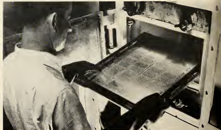
PHOTOSENSITIVE glass is processed at the new Corning Glass Works plant at Bradford, Pa. Each rectangle will be a printed circuit board for high temperature
