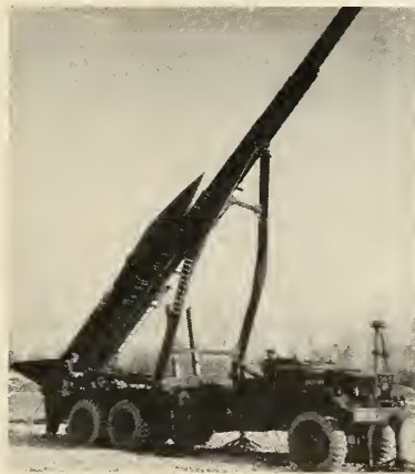
MISSILEMEN of U.S. Army's 1st Missile Command, Southern European Task Force, supervise an Italian Army cadre servicing the Honest John solid-fueled rocket.
