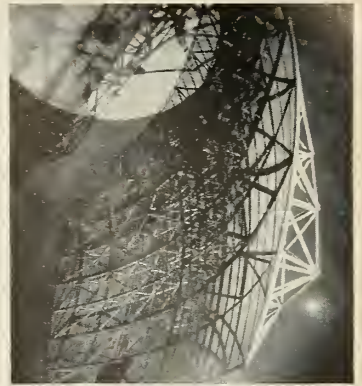
UNIQUE CONSTRUCTION DESIGN of the antenna system permits the inclusion of the latest 3-D height-finding techniques. Range, azimuth and height data can be automatically fed to a computer to form a composite picture of the air defense sector.
