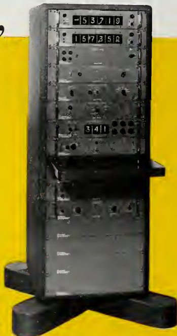
Multi-purpose digital system for measuring a variety of transistor parameters while the transistors are being subjected to environmental testing.
