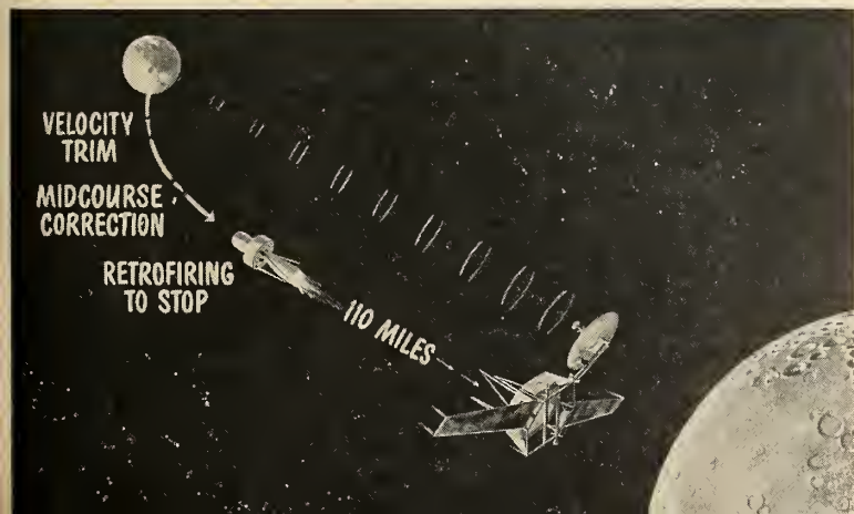
ARTIST’S CONCEPTION of how hard landing would be made on moon using Atlas-Agena vehicle with midcourse guidance correction.
