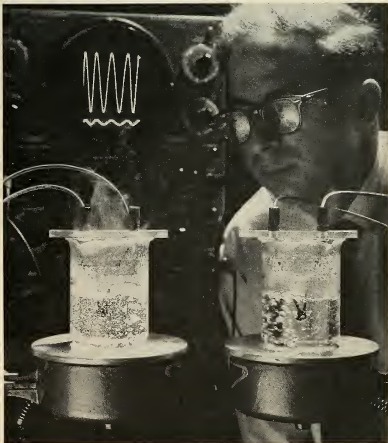
IN THIS DEMONSTRATION , thermistor at left displays its normal resistance at temperature of 100 degrees C. Thermistor, right, in boiling solution of ammonium chloride, displays resistance newly-developed roughly 20 times higher at about 112 degrees C.
