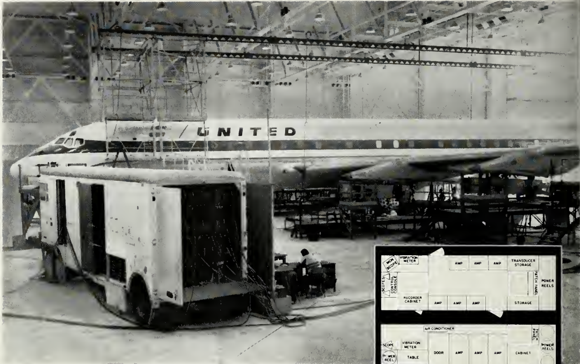
COMPLETE, COMPACT LAB—control center at forward end . . . six amplifiers in the center and patching panels with power reels at the rear.
