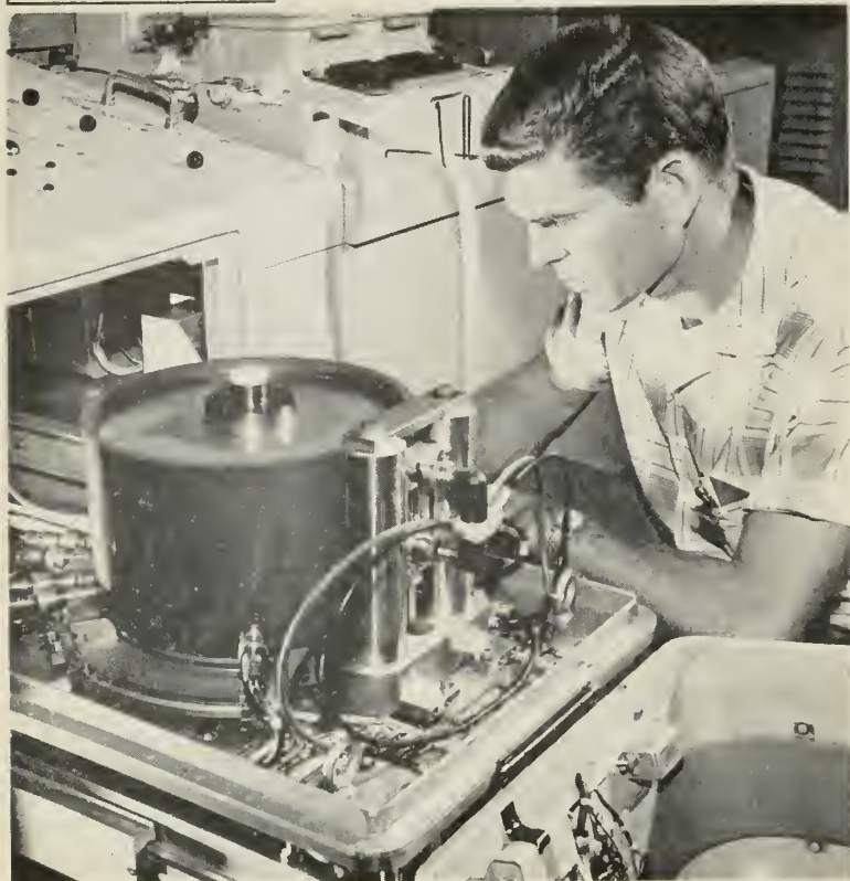
The first successful application of a moving pick-off head to a new, medium speed digital computer has been reported by engineers of Northrop Aircraft, Inc. With the device it is possible to record or read on 64 magnetic memory drum channels using only two pick-off heads. While the drum revolves at 1,800 rpm, the moving heads make one full up-down cycle every two seconds. Previously, 64 separated heads, one for each channel, were required, resulting in greater weight and complexity. Pick-off hid circuitry requirements, for example, have been reduced by over 95% by Northrop's new development.
