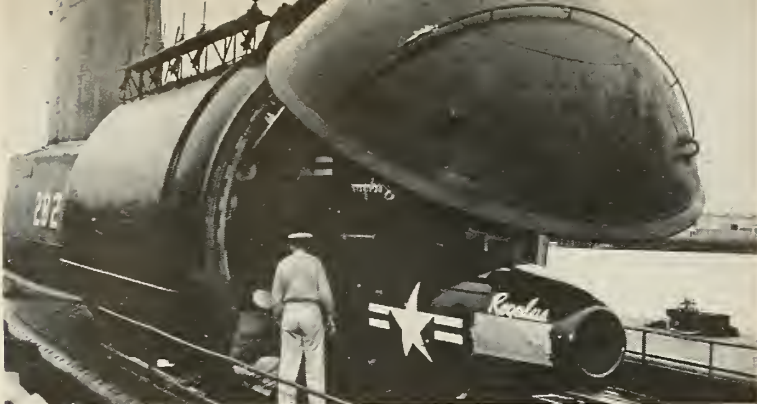
One bird slides easily from twin cocoon on submarine's deck while second missile waits for it to clear before rolling down and around to the ready.
