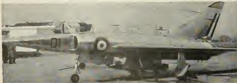
A MATRA air-to-air missile has been installed underneath the prototype of the Dassault Mirage, France's Mach 1.5 fighter prototype.
