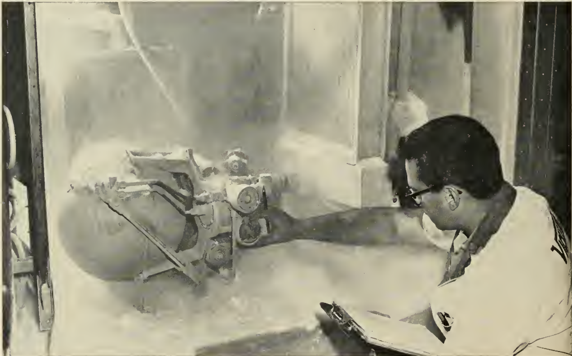
PUMPING UNIT AND CORE. Large airborne cooling system developed by Vickers' Aero Hydraulic Products division makes efficient use of 3M's FC-75 dielectric coolant to dissipate heat from electronic countermeasures equipment. Output pressure is required to be approximately 100 psi with fluid flow rates as high as 52 gpm. Operating range is from -65^{\circ}\text{F} to 210^{\circ}\text{F} . Pumping unit weighs 54 lb. dry and the heat exchanger core only an additional 20 lb. Shown below is part of the extensive testing program conducted by Vickers to prove out the new design. It included extremes of heat and cold as well as vibration, shock, attitude and other physical tests.
