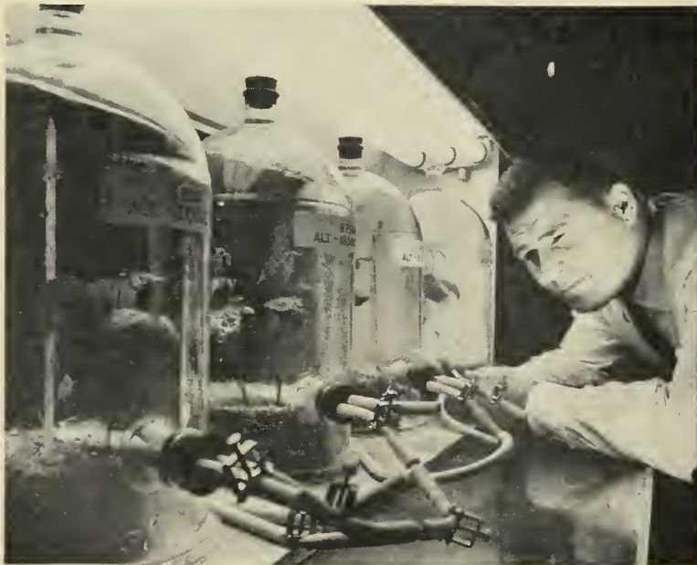
IF ASTRONAUTS are going to stay long on the moon, they may have to raise their own food. Anticipating such a need, Republic has turned to raising carrots, beets, snap beans and turnips in a low-pressure "lunar greenhouse."
