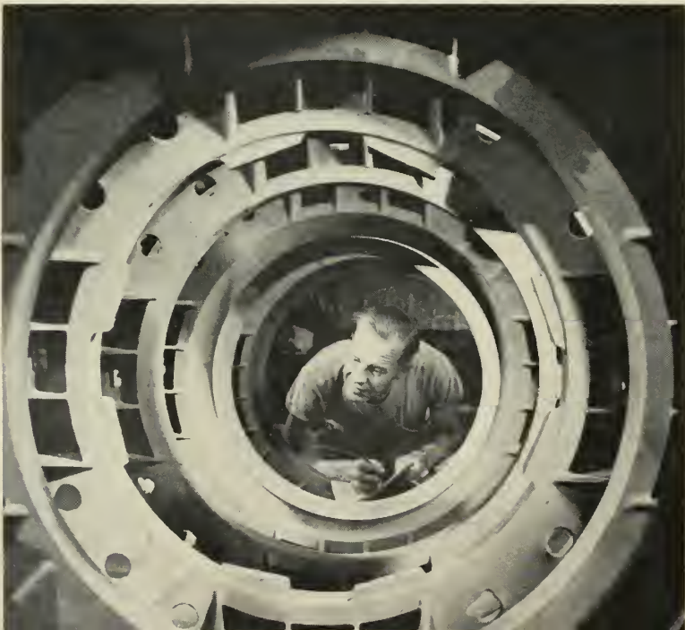
THESE COMPLEX structural steel castings have passed stringent inspections. Flaws permissible in normal castings would cause the rejection of these parts.
