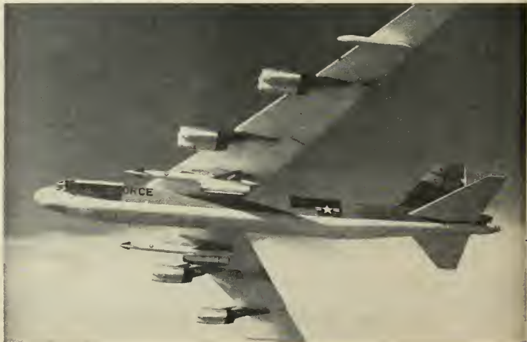
A FLYING launch pad, this Boeing B-52G Stratofortress can destroy three targets in one mission; two with the Hound Dog missiles under the SAC bomber's wings, and a third with the regular bombload.
