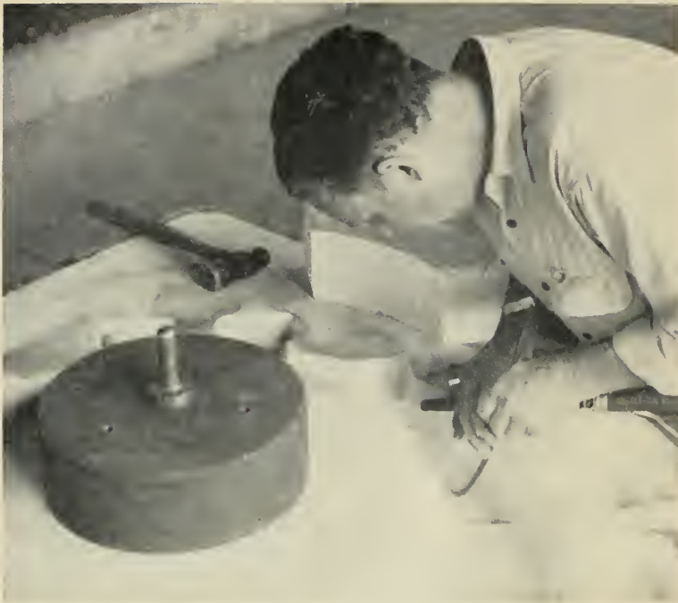
CORES ARE carefully set in specially prepared ceramic molds.
