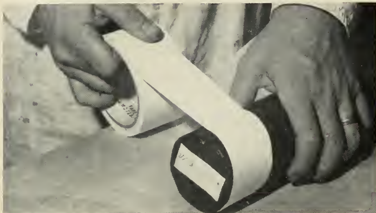
WRAPPING GLASS tape on solid propellant charge for Rocketdyne generator.
