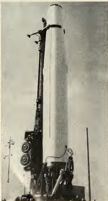
THE FIRST operational Thor IRBM fired Dec. 16 from Vandenberg AFB was minus the fins used on earlier missiles.
