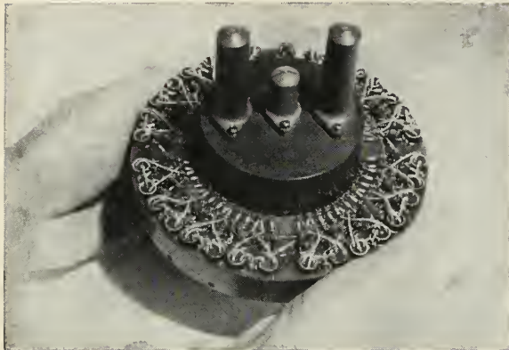
INSTRUMENTS THAT measured the two radiation belts during the flight of Pioneer III on Dec. 6-7. The two Geiger-Mueller tubes measured the intensity levels.
