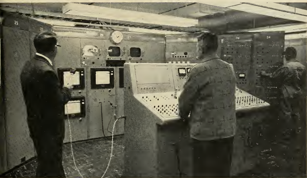
CONTROL CENTER from which Aerojet operates three static test stands for the Minuteman's solid rocket motors. The center uses the most advanced instrumentation equipment. Test results, monitored on 300 channels, can be available to the test engineer in less than four hours.
