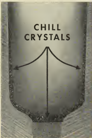
WHY FORGE? These Ladish Co. photos show how any casting forms from molten
