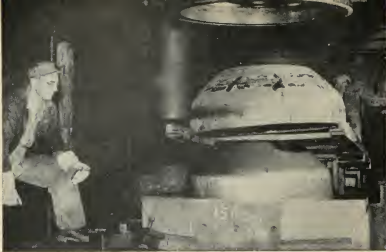
TITANIUM MOTOR CASING CLOSURE forged at the Wyman-Gordon—U.S.A.F. plant in North Grafton, Mass., weighs 441 lbs. and has 41.16" O. D.
