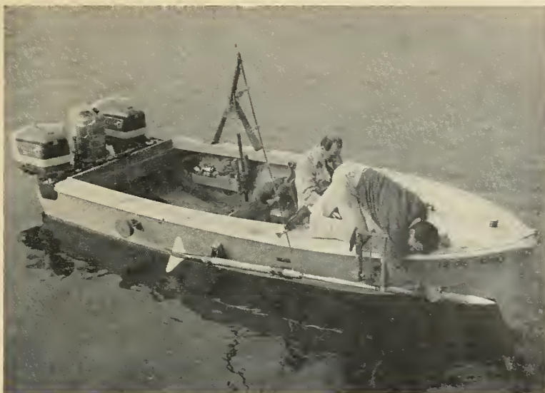
STREAMLINED TEST device is placed in water. Coating developed by U.S. Rubber has brought about 50% reduction in drag underwater.
