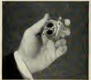
100,000 rpm turbine-driven alternator
