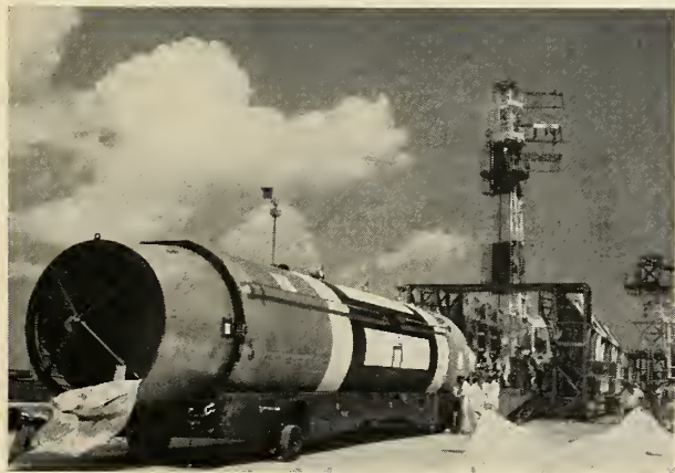
TRANSTRAINER vehicle, manufactured by North American Aviation, is used in transporting Titan from Denver to Florida on C-133 aircraft and then takes to the road for delivery to pad.
