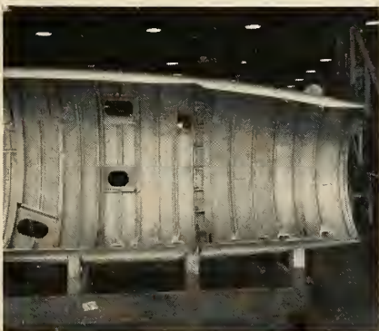
Access door on DC-8 engine assembly, fabricated entirely of titanium. Skin is .016" thick, ribs and longerons are .032" thick.
