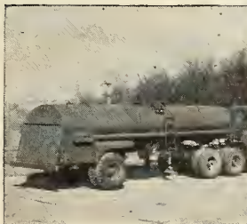
Water-alcohol fuel service unit for Redstone. Research, design testing and fabrication by Butler Contract Manufacture Division.
