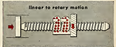
SCREW TRAVELS: When rotary motion is applied to the b/b nut, the screw glides along its longitudinal axis on rolling steel balls, converting rotary force and motion to linear force and motion with unprecedented efficiency.
