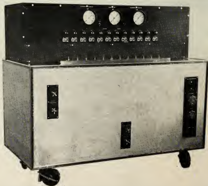
PRESSURE CABINET of Autocal contains six standard transducers, a standard transducer selector and servo system, manifold connections for 12 test transducers, plus voltage power supplies and other components.
