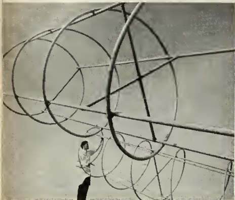
Doppler radar antenna picks up data on electron density in space 50 miles up and out.
