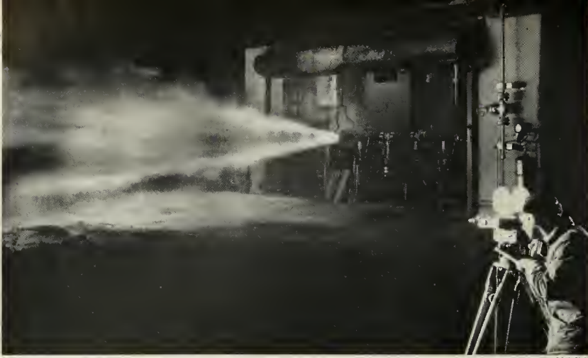
CAMERA HELPS RECORD the firing of a 5,000-pound thrust high-energy fuel rocket.
