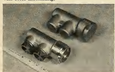
Below: Titanium alloy ejector breech, before and after machining.
