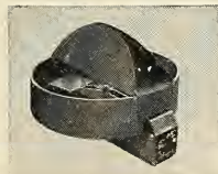
MODEL B78 Accommodates test objects up to 25 pounds; 1200 G-pounds max.
