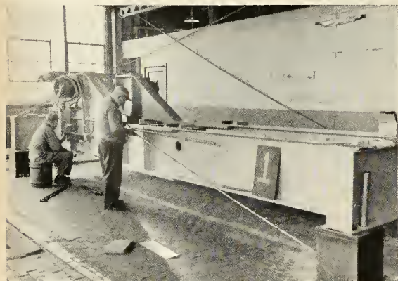
3 Completed base—sand blasted, and painted—is moved to final assembly where lines and wiring are installed.
