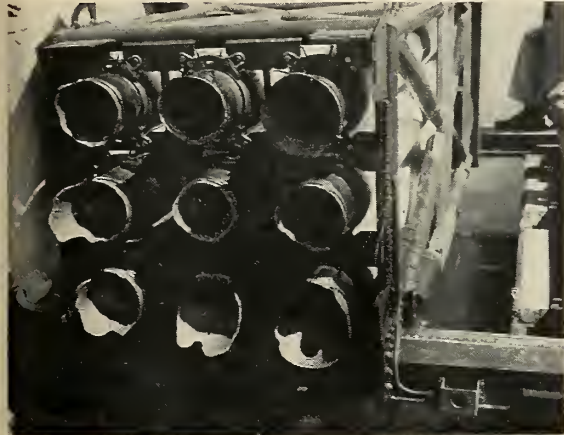
NOZZLE END of Grand Central Javelin rockets after Narmco fin test. Note nozzle erosion towards center of cluster in "hot spot" areas.
