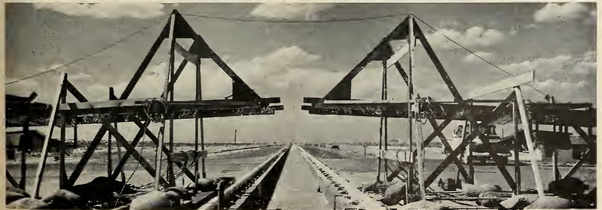
THESE RACKS were used to hold quart lamp heaters (which simulated aerodynamic heating) at the start of the sled's run.
