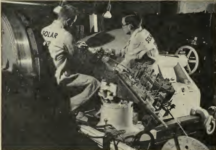
AFTER GRINDING, while still on the lathe, the turning chamber is wrapped with strips of ribbon-wrap and copper braze alloy fed out by Solar technicians from a spool geared to lathe's revolutions.
