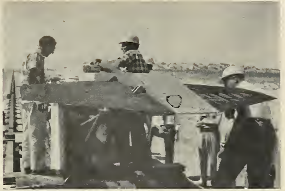
SLED AND FINS are re-checked after run. Test program included highest thrust operation (about 270,000 lbs.) ever attempted at Holloman track. Titanium fin (right) shows some indication of high loads. No material was ablated from either fin. Velocity of sled was approximately 2400 ft. per sec. (1636 smph). Vehicle weighed 6500 lbs. and required a run of 27,000 ft. AFMC sled was designed and built by Coleman Engineering Co. Power is nine 30,000-lb. thrust Grand Central Javelin rockets.
