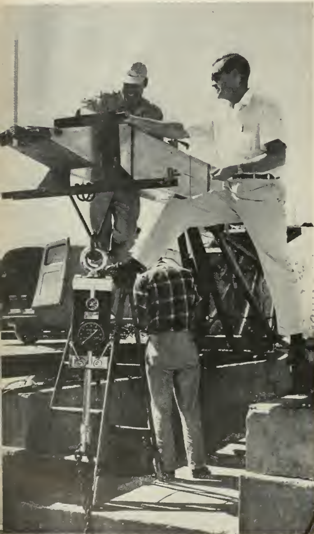
PYLON for fin mounting to avoid aerodynamic interface with the sled was fabricated by AFMDC personnel to Narmco recommendations. During static tests, loads were applied to the pylon at the predicted center of pressure under maximum fin loads. Procedure enabled determination of load-deflection curves for pylon and to proof-load pylon and sled in a structural check.
