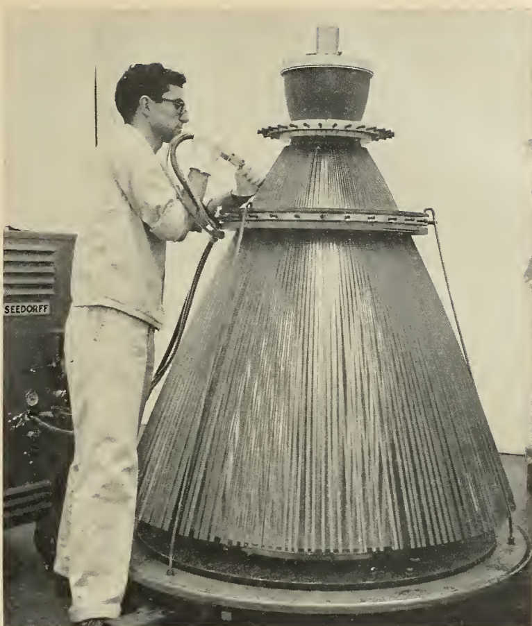
ABOUT 100,000 spot welds are applied to channels in a specific pattern to insure close fit and to hold dimensional and configuration requirements of the chamber being fabricated for NASA.
