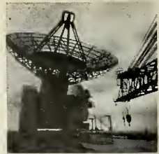
COVER: This large antenna is part of radar network on Army's missile tracking ship SS AMERICAN MARINER.
