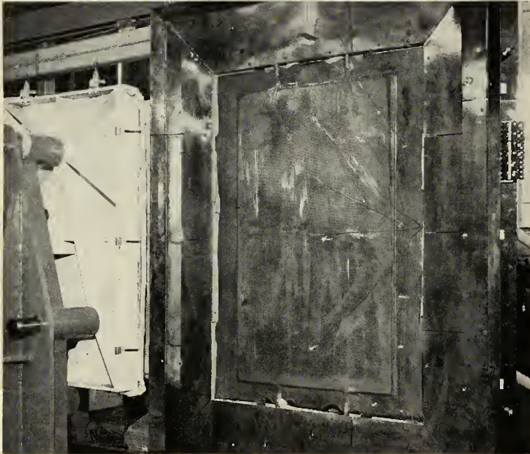
THERMOCOUPLES ATTACHED to the outer skin of a brazing envelope containing a stainless steel honeycomb sense temperature variations and instantly apply precise heat corrections during the brazing cycle.
