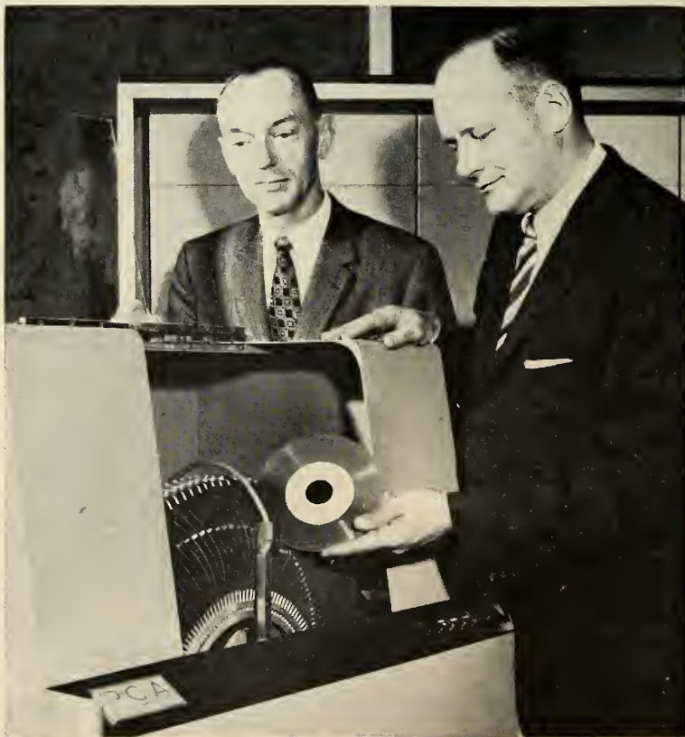
MAGNETIC MEMORY discs of the RCA 301 data processing system are examined by two RCA vice presidents, T. A. Smith, Industrial Electronic Products Div., and D. H. Kunsman, Electronic Data Processing Div. This is the first data processing system to use magnetic discs—similar to 45-rpm records—for its memory "storehouse"; it also can use magnetic tape on reels.
