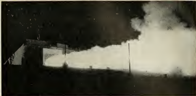
TESTING OF the Thiokol booster engine used in Nike-Zeus. The solid-propellant engine delivers 450,000 pounds of thrust in about four and a half seconds.
