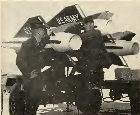
THREE HAWKS ready to go are mounted on mobile launcher at White Sands Test Range. They can be fired in rapid succession.
