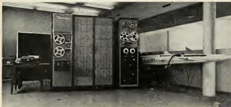
CURTISS-WRIGHT'S DEMON checks out a Nike-Ajax. DEMON—along with Nortronics' NORSCAN—represent solid state technology for automatic checkout. (Fig. 1)
