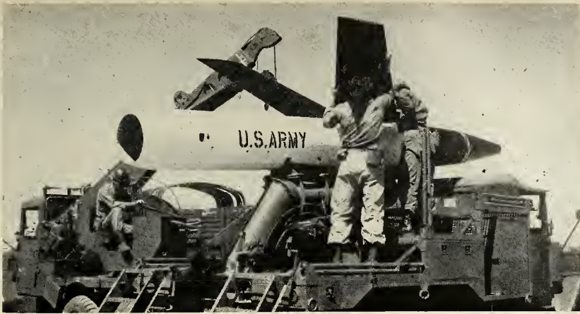
LACROSSE , the Army's new surface-to-surface tactical missile, is mounted and ready for launching from standard 2½-ton truck.
