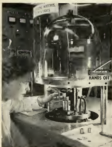
HAWK RATE GYRO is silver brazed at 1300°F in two minutes under controls.
