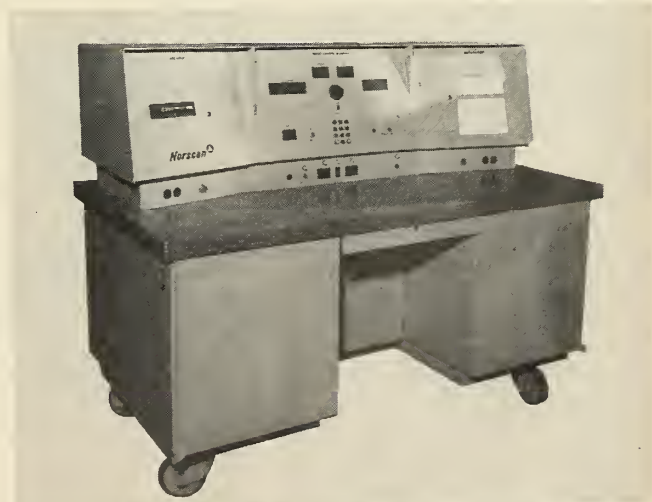
PROTOTYPE CONSOLE of NORSCAN. Magnetic drum memory device in system has one-half million information bits capability. (Fig. 4)
