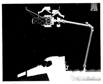
PLAID Computer Illustrations From top down: 1) After the truss assembly has been constructed, Kathy Thornton grabs and maneuvers the Multipurpose Experiment Support Structure with the help of robot arm operator Bruce Melnick. 2) Next, she and Tom Akers attach the MPESS to the truss with "legs." 3) The following day, Melnick drives Rick Hieb and
