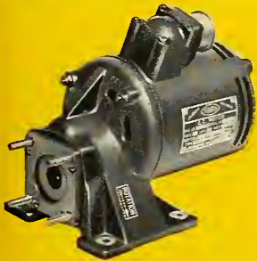
Type: D-899 400 cycle 3 phase AC Motor. Weight: 11.25 lbs. Volts: 200 volts. Load: 2.75 hp continuous output. RPM: 3140 rpm output at gear box. Power factor: 83%. Overall efficiency: 76% for entire unit. Meets Military Specification MIL-M-7969A (ASG).
