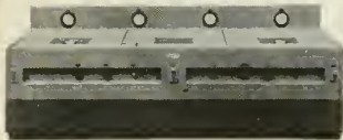
TUBE TEST MACHINE. CAPACITY 16 GPM AT 500 PSI FOR FILLING AND BLEEDING TUBES, APPROXIMATELY 0.10 GPM TO 10,000 PSI FOR STATIC TESTING. SAFETY COVERS WILL NOT OPERATE WHEN MANIFOLD IS PRESSURIZED.
