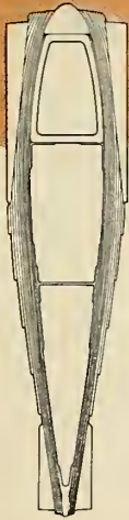
Cutaway cross-section of inboard half of the XH-40 rotor blade showing how the extrusions, machined ports, and contoured aluminum sheets are bonded with Narmco Metlbond 4021.
