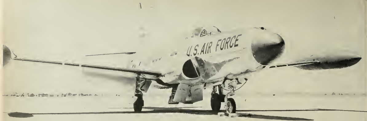
The F-94C aircraft used in parabolic flight to obtain reduced gravity states.
