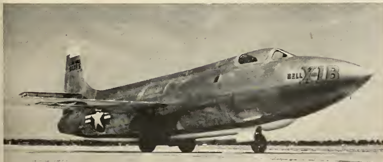
The X-1B was designed to test the effects of aerodynamic heat on aircraft structures.
