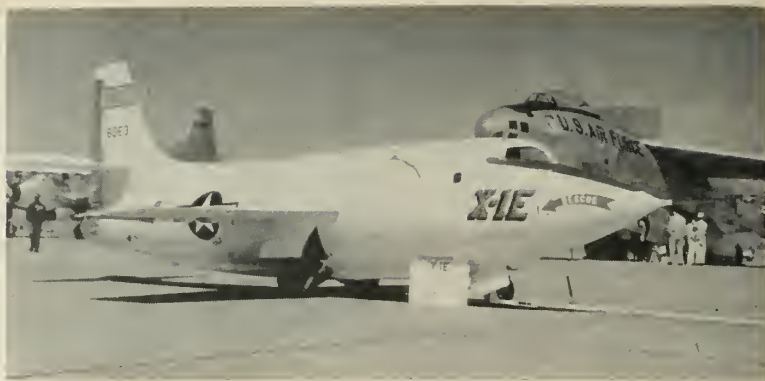
The X-1E was the last of the X-1 series. It investigates high speed heat problems.
