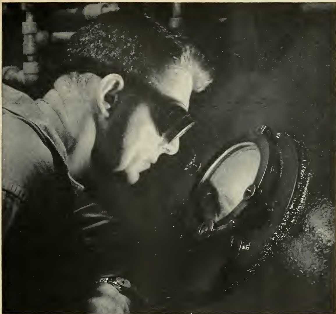
Utica technician viewing a meltdown of Udimet 500—a new vacuum melted alloy in the high temperature field.
