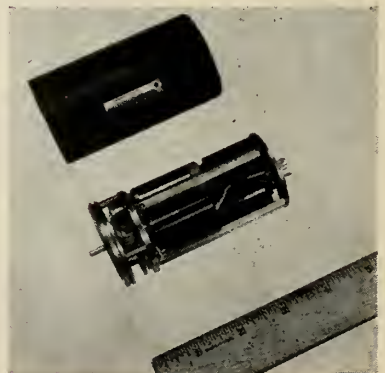
Fig. 2. Synchro-type servo-repeater module.
