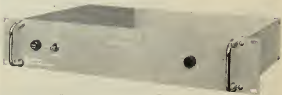
Power module for power and reference voltages and flexowriter module for sensing meter balances and operating typewriters.
