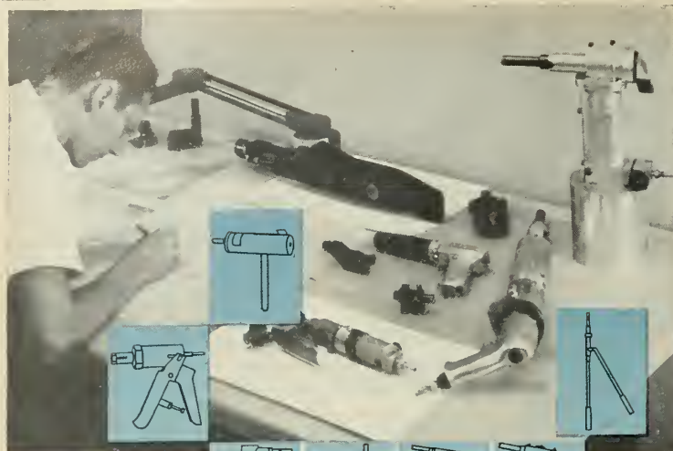
Prototypes of new special tools for installing Cherry Blind Rivets and Lockbolts are shown in the Cherry Research and Development Department.
