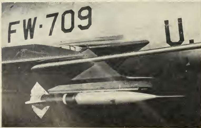
DUAL-THRUST rocket motor powers C-W's expendable SkyDart TDU-12/B drone. Supersonic vehicle costs about $2000 per copy.
