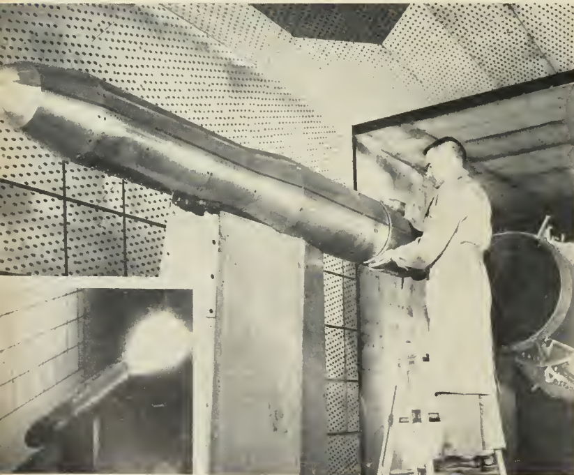
TITAN ICBM, in 11.5%-scale model, is installed for transonic test runs in the 16-foot test section of the Propulsion Wind Tunnel at Tullahoma. Inset is a frame from a motion picture film showing the missile with its rocket operating during a test run at the 10-year-old Arnold Engineering Development Center.
