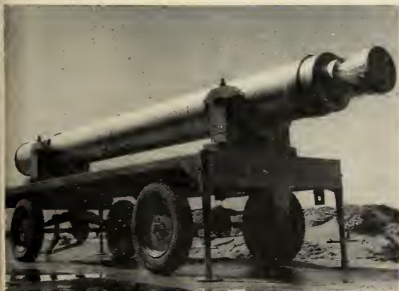
K-420 IS LARGEST solid motor in Kappa project, studied at the University of Tokyo. Its diameter is 420 mm, length is six meters. Thrust is 10 tons, and duration is 15 sec.
