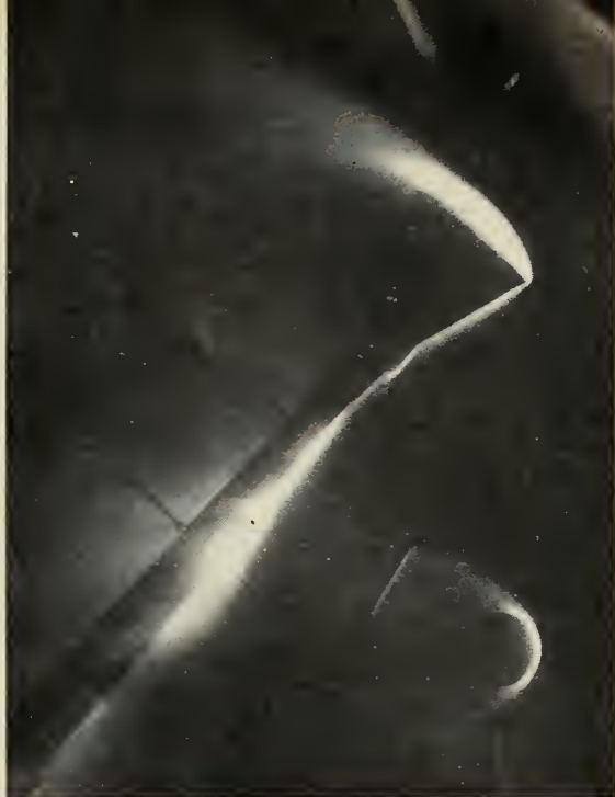
HYPERSONIC airflow is shown striking Mercury capsule at 50° angle of incidence. Mach 20 airflow became incandescent during test lasting 0.1 second, which determined stability and heat transfer characteristics.
