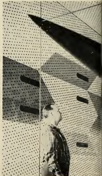
FULL-SCALE flight-type Sergeant missile, about 30' long, is installed for transonic test program in the 16' Propulsion Wind Tunnel at AEDC. Such tests illustrate
