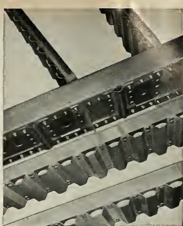
WING SPARS, FRONT AND REAR, HAVE SPAR CAPS ATTACHED TO WEB SECTIONS WITH HS92 PINS, A286 ALLOY, HEAT TREATED TO 95,000 PSI MINIMUM SHEAR. HS60M COLLARS ARE USED.
