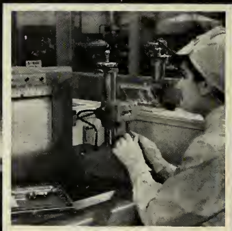
Comparator measures dimensions to one-millionth of an inch. One of many pieces of ultra-precision equipment in the New Departure instrument/minature ball bearing laboratories.
