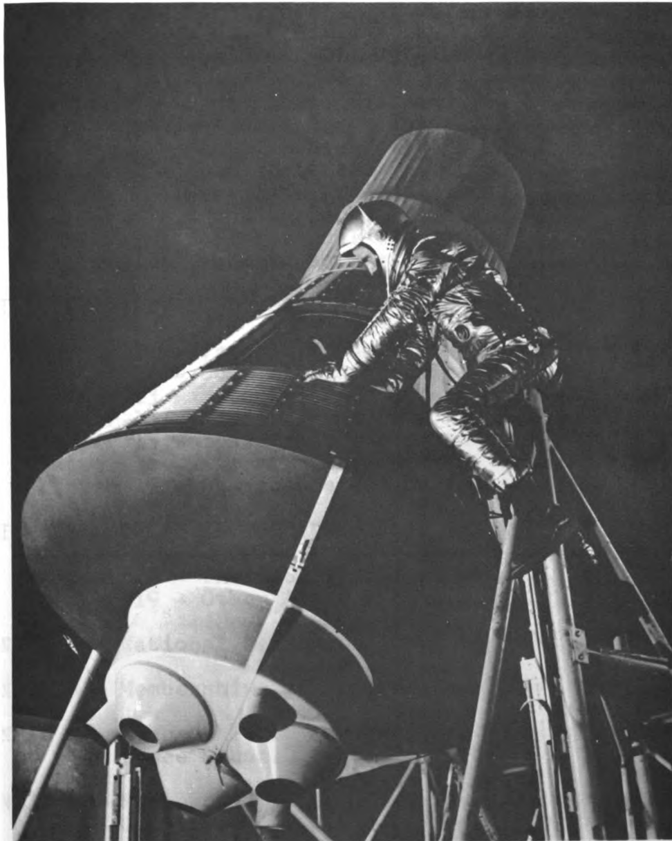
Wearing a full pressure suit of the type being developed for use in the NASA Project Mercury program, an engineer inspects a full-scale model of the Project Mercury capsule being constructed by McDonnell Aircraft Co., St. Louis, Mo. At lower left is the mounting for retrorockets which, when fired in the direction of the capsule's flight, will retard its speed so that it will reenter the earth's atmosphere for recovery. (See Project Mercury .)
