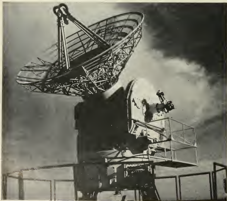
ANTENNA for new AN/FPS-16 instrumentation radar units at White Sands. It is considered the first radar designed originally for supersonic missile tracking.
