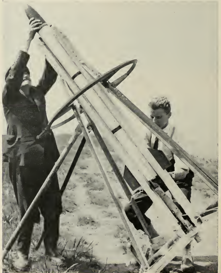
ROCKET BUFFS ready the postal rocket for firing. It will deliver postcards and letters to North Sea islands where it will land by parachute and be returned.
