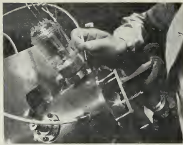
PROTOTYPE of Minneapolis-Honeywell's electrically-suspended gyro. Beryllium rotor is suspended in a vacuum.
