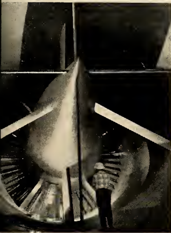
VARIABLE STATOR vanes in transonic circuit of the propulsion wind tunnel help control the airflow from three-stage compressor at Arnold.
