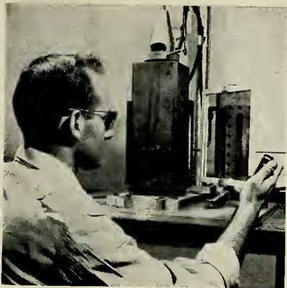
PHIL FERRIS watches the burning of a new liquid monopropellant inside a high-pressure bomb with Lucite viewing windows.
