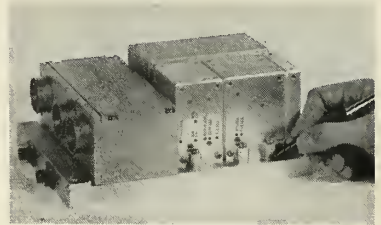
ASCOP K-SERIES Mixed Input Multicoder, assembled to fit missile test requirements. Dual commutator is on the left.
