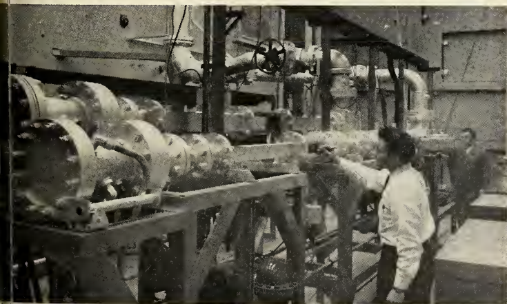
FLOW TUBES for investigating shock-wave interaction and influence of flow on detonation wave characteristics.
