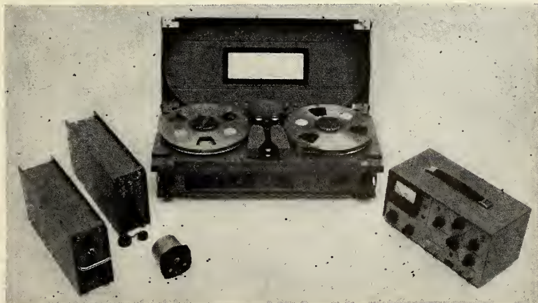
A COMPLETE airborne or mobile type AR-200 magnetic tape recorder system is shown from left to right: power converter, electronics box, remote control unit, AR-200 tape transport, and test unit. Design includes an alternate-opening transport cover permitting opening from front or back or complete removal. Total weight: 90.5 lbs.
