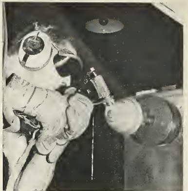
TUNGSTEN IS applied to missile nose cone with torch, after being drawn into the arc in powder form.
