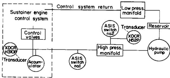
FIGURE 1-14.—Launch-vehicle hydraulic diagram.
