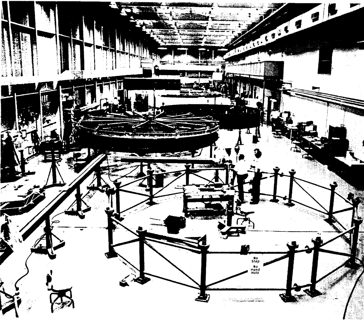
ASSEMBLY AREA—Saturn IB launch vehicle instrument units are shown in various stages of assembly at IBM's Space Systems Center in Huntsville, Ala. At the far end of the bay is the unit for the first Saturn IB, the Apollo 201 mission. IBM has a $175 million contract with Marshall Space Flight Center for building and testing 27 instrument units—12 for Saturn IB and 15 for Saturn V.
