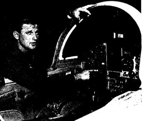
Project Manager Scott Reagan showed off Flight Crew Operations' prototype for upgrades to NASA's fleet of T-38 astronaut training aircraft. The "glass cockpit" is expected to make flying safer with weather and other flight information upgrades.
