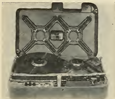
TAPE RECORDER stores 1500 bits per inch on each of 16 tracks. Note flangeless reels. Overall dimensions are 6 \frac{3}{4} by 18 by 26 inches.
