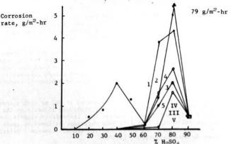
Corrosion rates at room temperature in 100-hr test in sulfuric acid of various concentrations (Arabic numerals) and 164-hr test in 80% sulfuric acid (Roman numerals) 1 and I - unalloyed titanium; 2 and II - 1% platinum alloy; 3 and III - 2% platinum alloy; 4 and IV - 1% palladium alloy; 5 and V - 2% palladium alloy.
